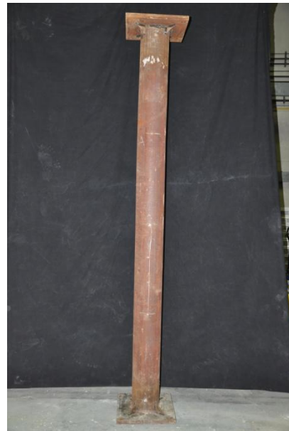
Figure D.28 – Deformed shape of column A28 219-RING-PC-70%-Khigh.
