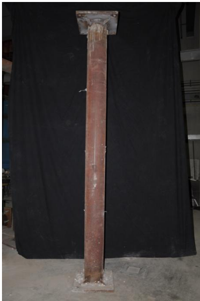
Figure D.26 – Deformed shape of column A26 219-TOT-PC-70%-Khigh.
