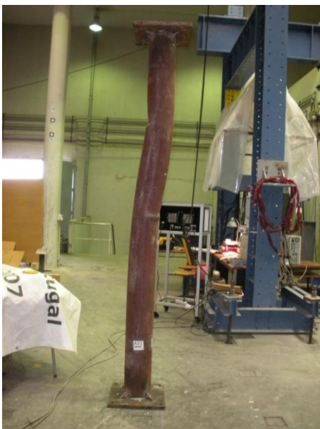
Figure D.10 – Deformed shape of column A10 219-70%-Klow.
