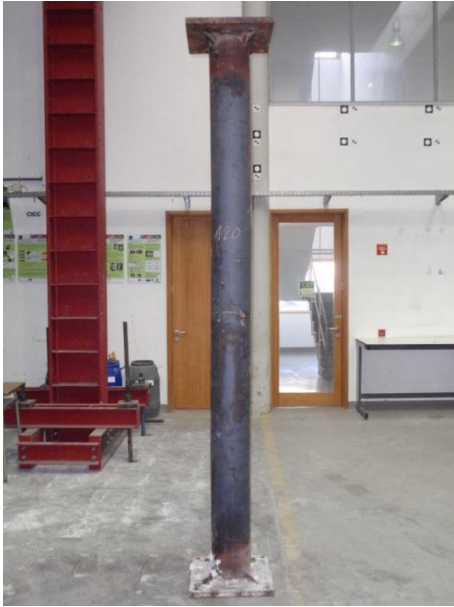
Figure D.17 – Deformed shape of column A17 219-TOT-RC-30%-Klow.
