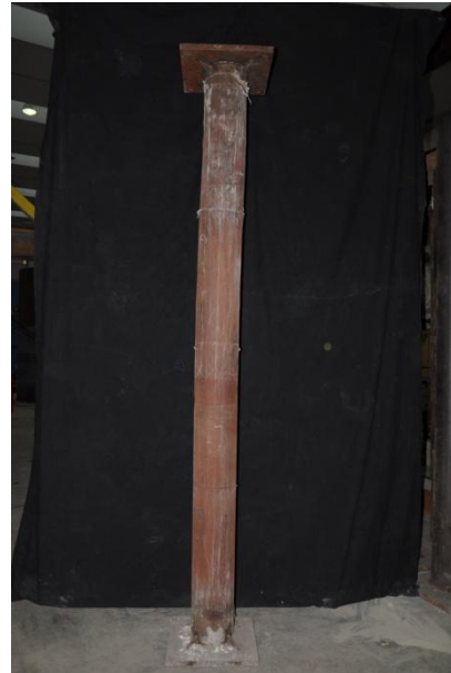
Figure D.39 – Deformed shape of column A39 219-RING-RC-30%-Khigh-
