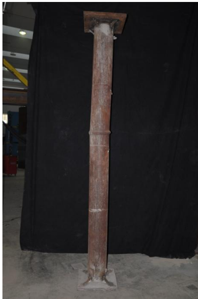
Figure D.29 – Deformed shape of column A29 219-RING-RC-70%-Khigh.
