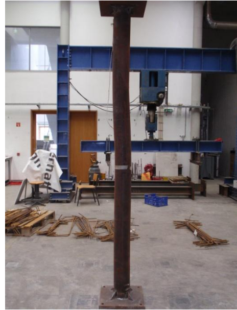
Figure D.15 – Deformed shape of column A15 168-30%-Klow.
