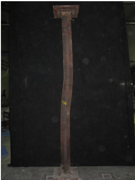
Figure D.14 – Deformed shape of column A14 168-RING-RC-30%-Klow.
