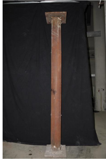
Figure D.27 – Deformed shape of column A27 219-TOT-RC-70%-Khigh.
