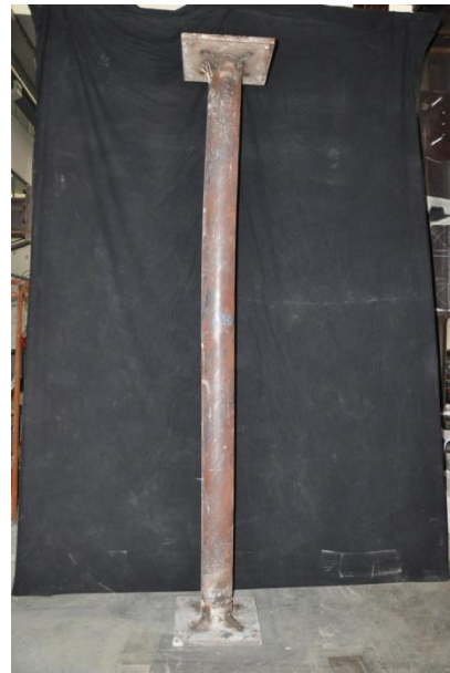
Figure D.23 – Deformed shape of column A23 168-RING-PC-70%-Khigh-
