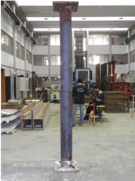
Figure D.37 – Deformed shape of column A37 219-TOT-RC-30%-Khigh-
