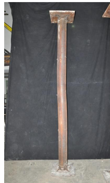
Figure D.24 – Deformed shape of column A24 168-RING-RC-70%-Khigh-
