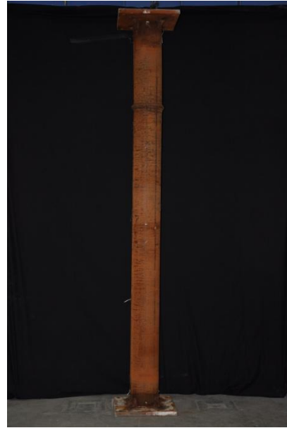
Figure D.19 – Deformed shape of column A19 219-RING-RC-30%-Klow.
