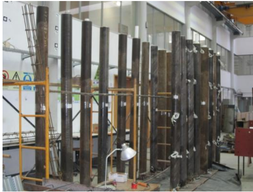
Figure 3.17 – Columns before the casting
