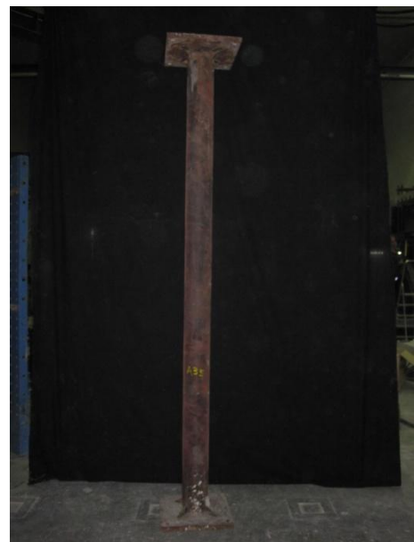
Figure D.12 – Deformed shape of column A12 168-TOT-RC-30%-Klow.
