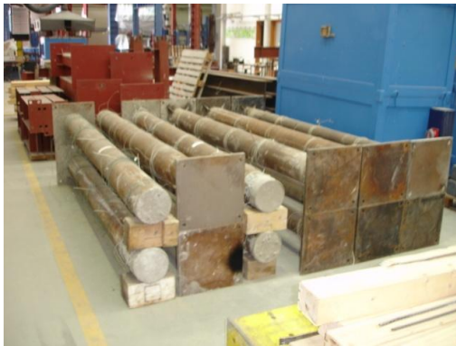
Figure 3.18 – Curing of the CFCH columns
