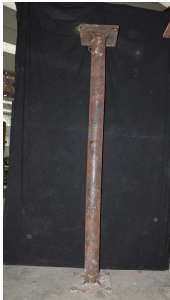
Figure D.33 – Deformed shape of column A33 168-RING-PC-30%-Khigh.
