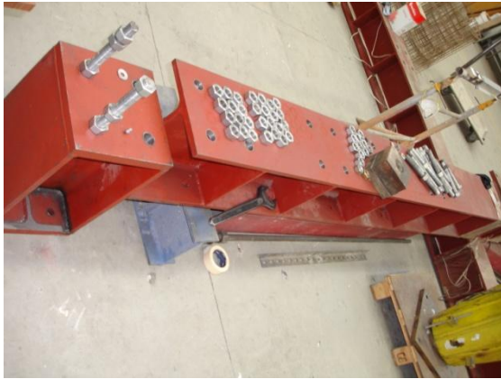
Figure 3.1 – Restraining steel beams and M27 threaded rods
