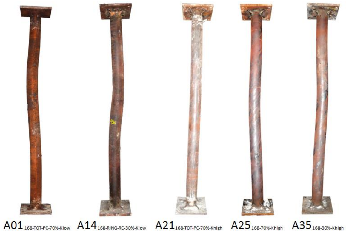
Figure 3.49 – Deformed shape of tested columns.
