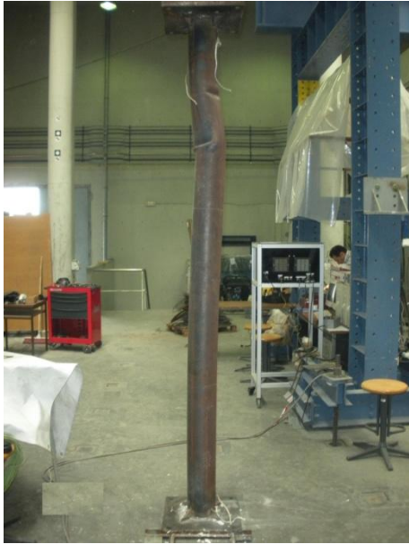
Figure D.5 – Deformed shape of column A05 168-70%-Klow.
