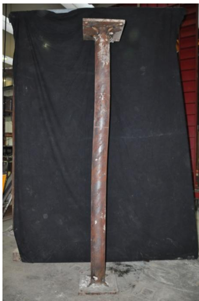
Figure D.34 – Deformed shape of column A34 168-RING-RC-30%-Khigh.
