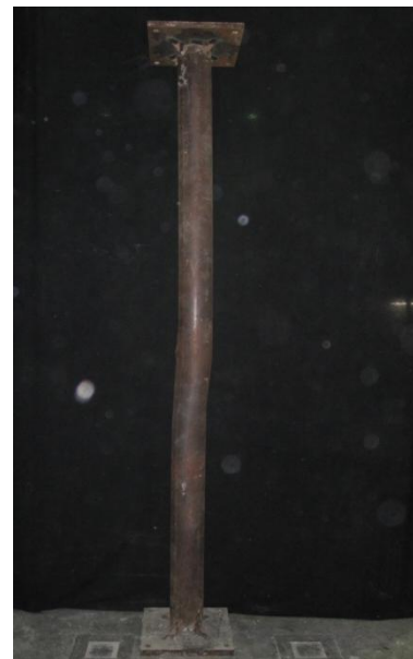
Figure D.4 – Deformed shape of column A04 168-RING-RC-70%-Klow.
