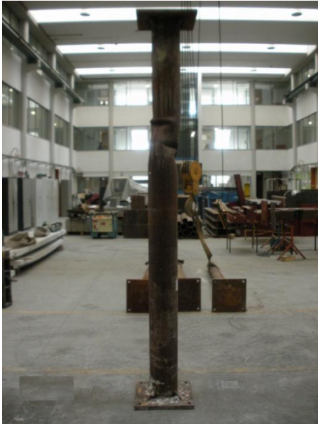
Figure D.9 – Deformed shape of column A09 219-RING-RC-70%-Klow.
