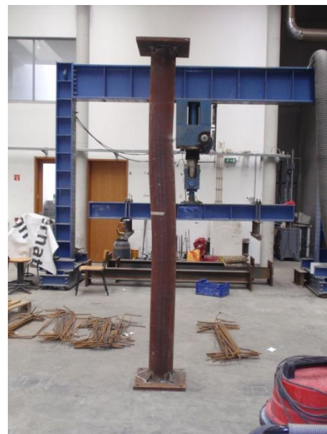
Figure D.20 – Deformed shape of column A20 219-30%-Klow.
