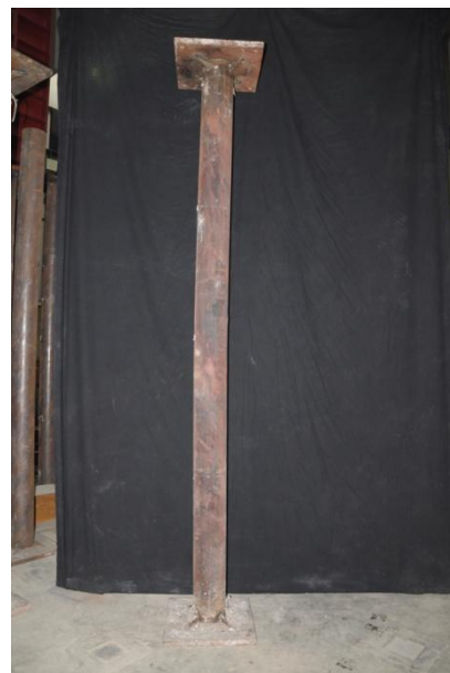
Figure D.32 – Deformed shape of column A32 168-TOT-RC-30%-Khigh.
