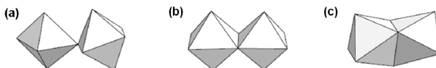
Figure 4-3 Different assemblies of union between two octahedral units in a POM (a) vertice, (b) edge and (c) share corners.
