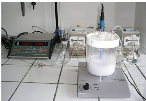
Figure 8-7 Illustration of the co-precipitation at constant pH set up employed in this thesis.
