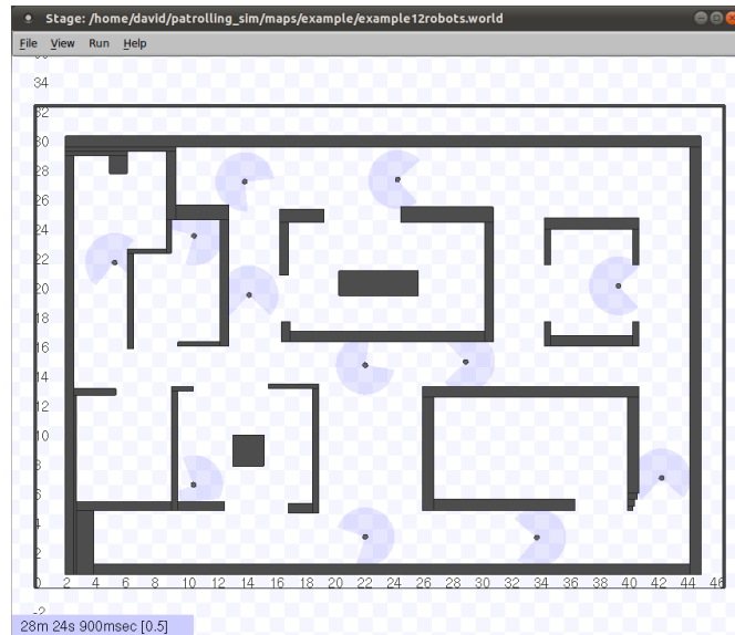
Figure 3.5: Snapshot of a Stage Simulation with 12 robots in Map B.
