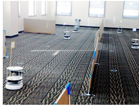
(d) A team of Turtlebots from the center for Robotics and Intelligent Machines at Georgia Tech Research Institute [Pippin et al., 2013].
