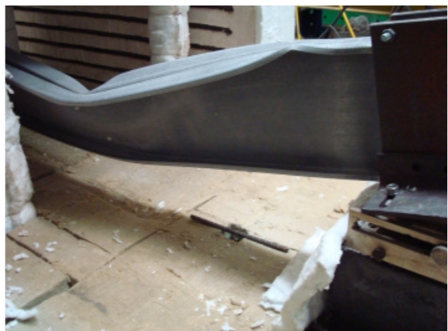
Figure F.18 – Back views of the failure mode of the specimen B-I_2
