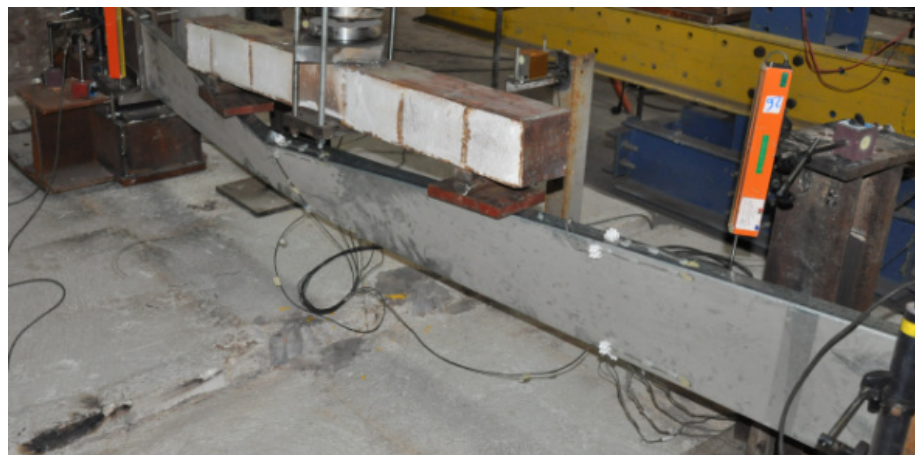
Figure 3.31 – Failure modes of the test beam B-I_3 at ambient temperature
