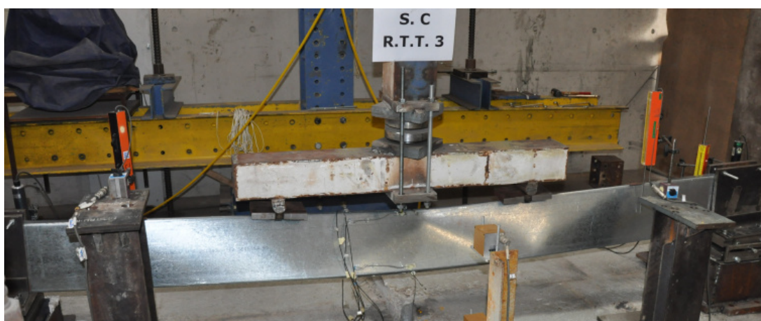
Figure 3.30 – Failure modes of the test beam B-C_3 at ambient temperature
