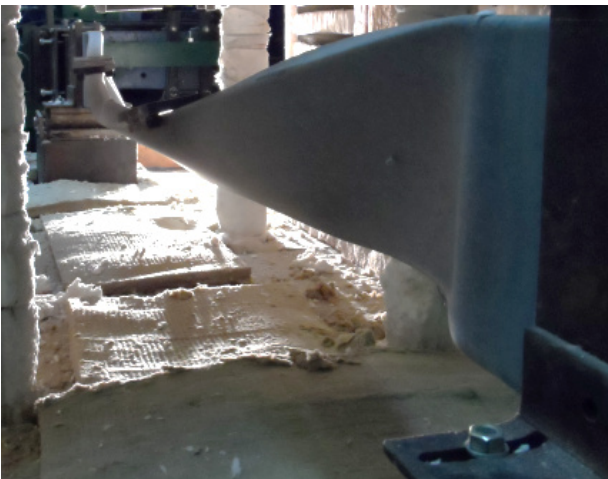
Figure F.77 – Lateral views of the failure mode of the specimen B_ka+kr-C_1
