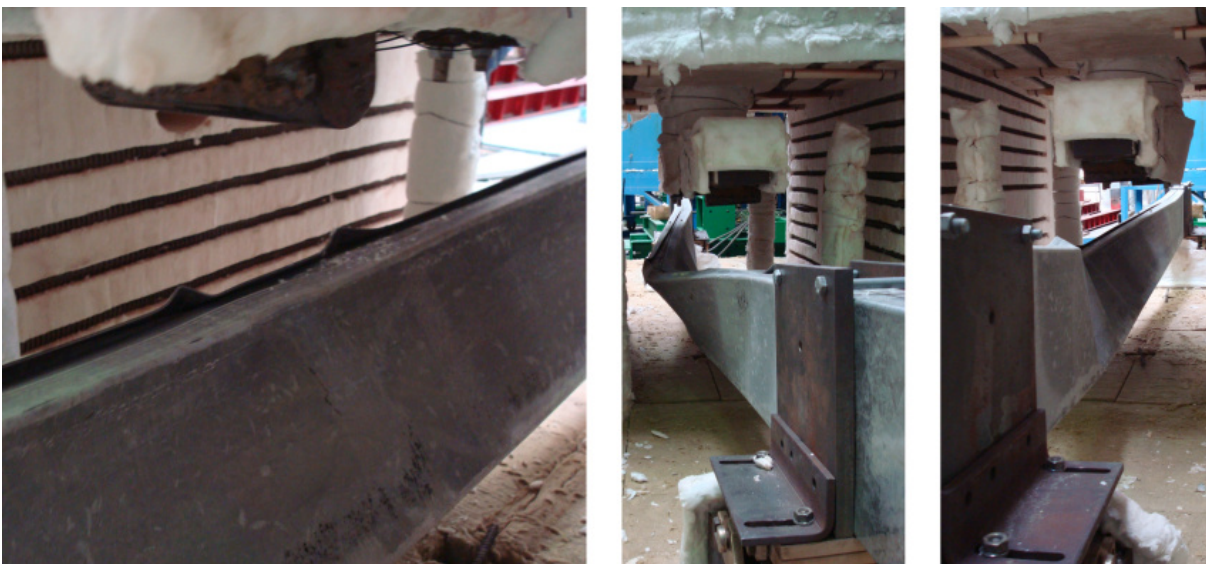
Figure 3.37 – Failure modes of the test beam B-2R_2 under fire conditions
