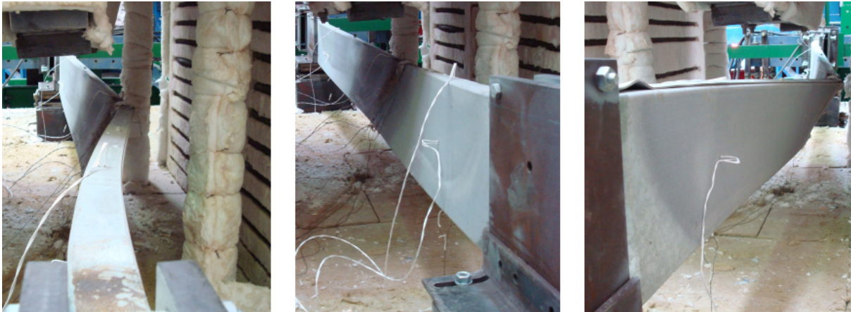
Figure F.67 – Lateral views of the failure mode of the specimen B_ka-R_3
