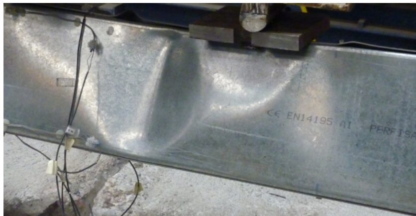
Figure B.26 – Detail view of the failure mode of specimen B-R_3
