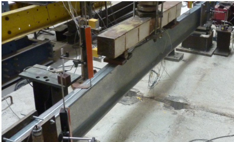
Figure B.15 – Front view of the failure mode of specimen B-I_3
