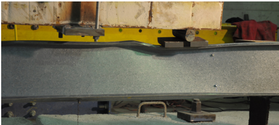
Figure B.11 – Detail view of the failure mode of specimen B-I_1
