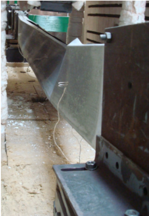
Figure F.70 – Lateral views of the failure mode of the specimen B_ka-2R_1
