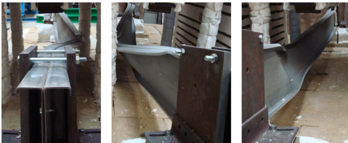
Figure F.15 – Lateral views of the failure mode of the specimen B-I_1
