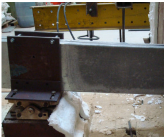
Figure F.36 – Back views of the failure mode of the specimen B-2R_1
