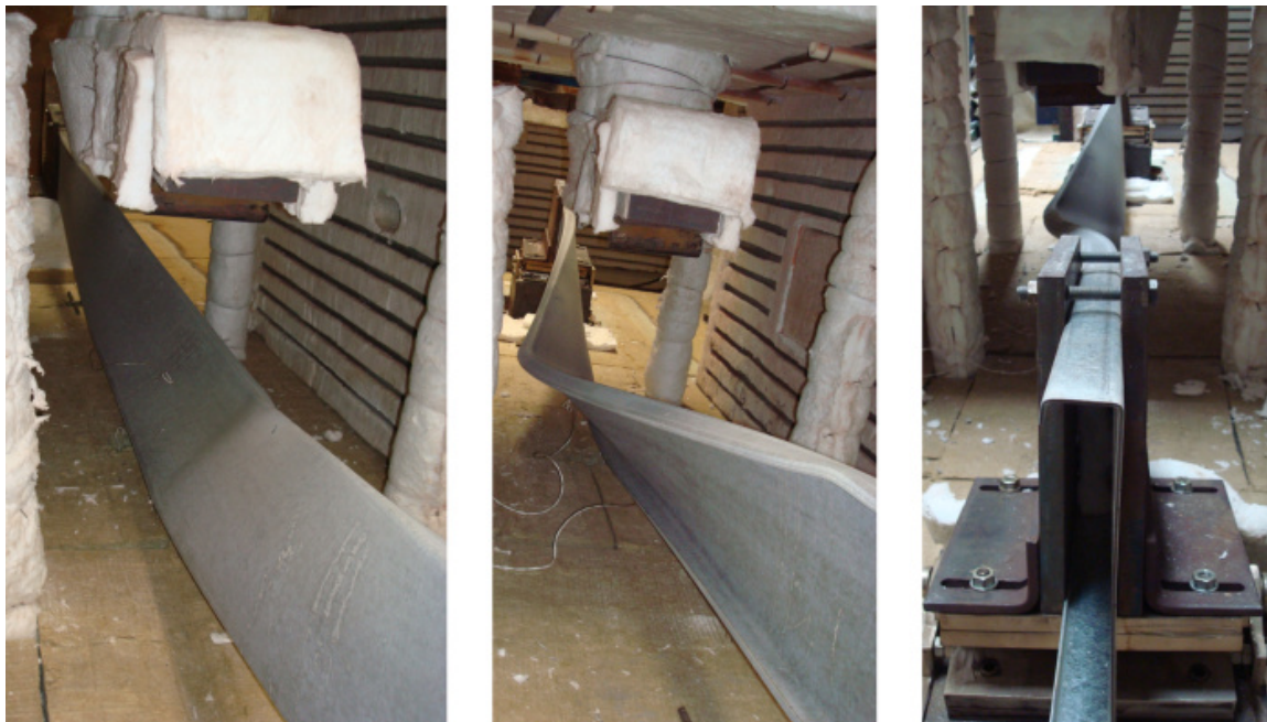
Figure 3.34 – Failure modes of the test beam B-C_3 under fire conditions
