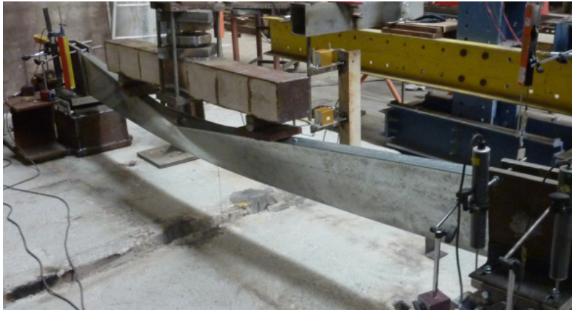
Figure B.19 – Back view of the failure mode of specimen B-R_1
