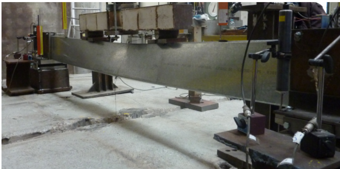
Figure B.2 – Back view of the failure mode of specimen B-C_1
