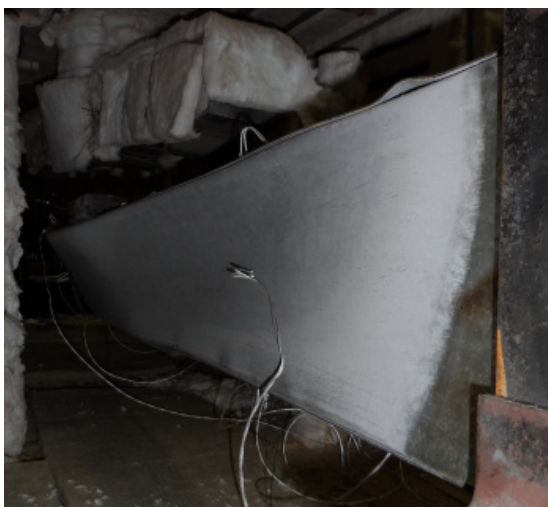
Figure F.90 – Lateral views of the failure mode of the specimen B_ka+kr-R_1
