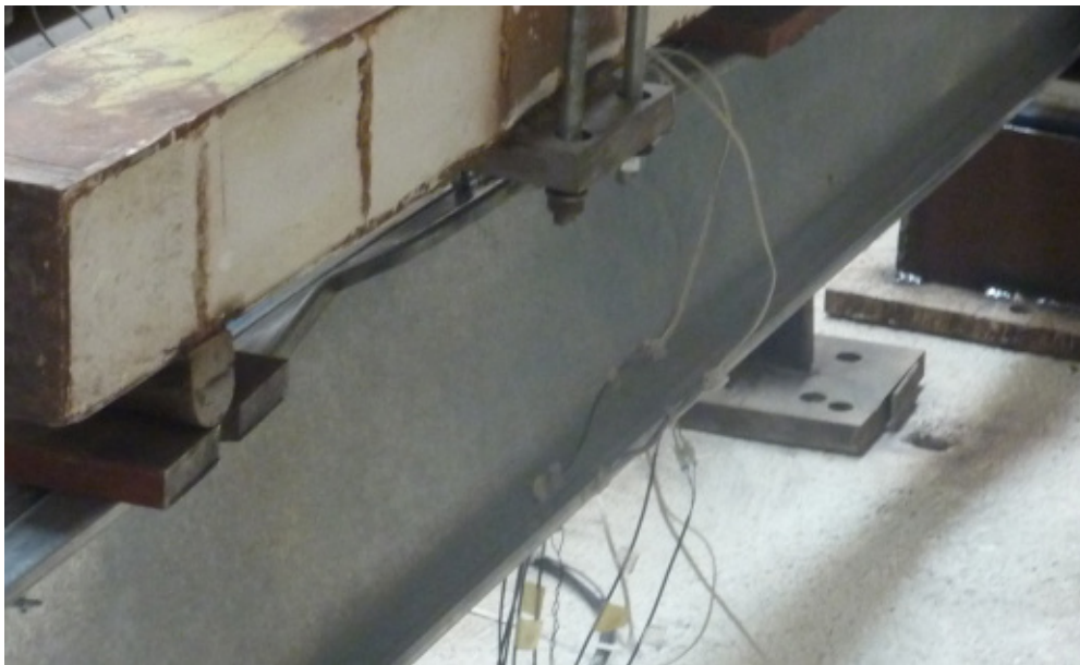
Figure B.17 – Detail view of the failure mode of specimen B-I_3
