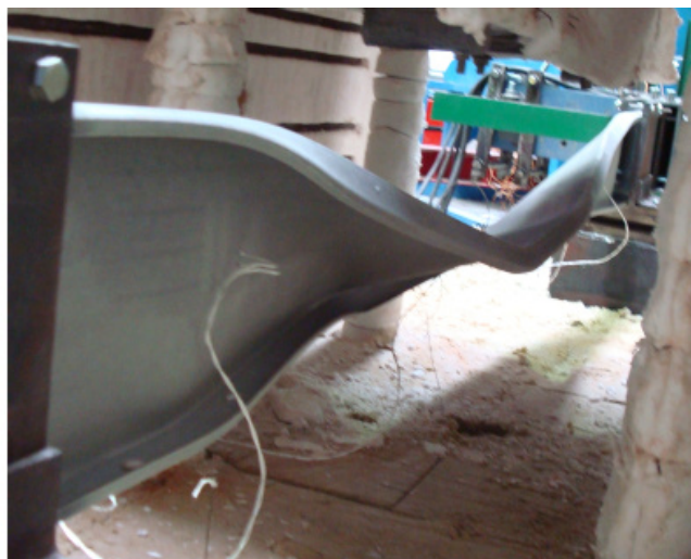
Figure F.53 – Lateral views of the failure mode of the specimen B_ka-C_2
