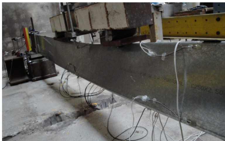
Figure B.5 – Back view of the failure mode of specimen B-C_2
