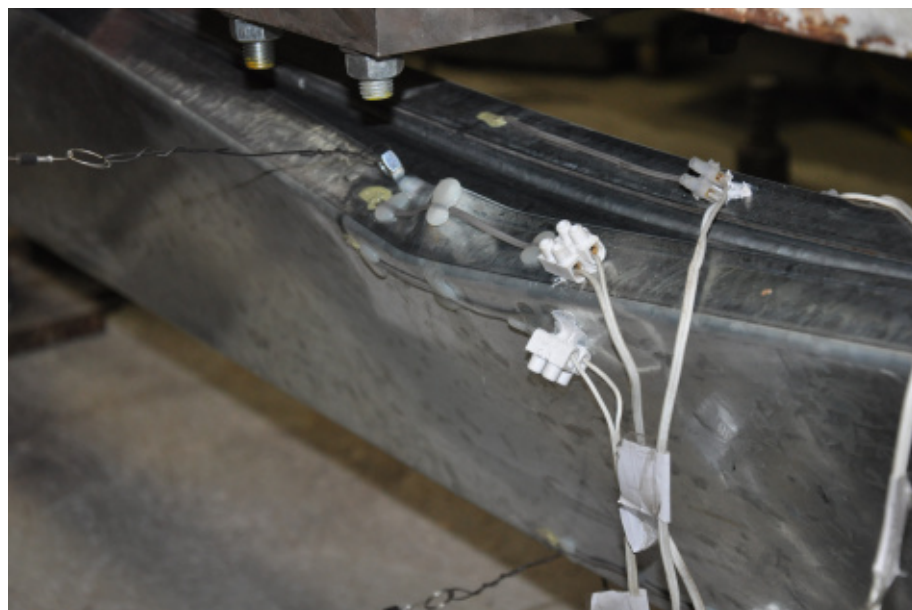
Figure B.35 – Detail view of the failure mode of specimen B-2R_3
