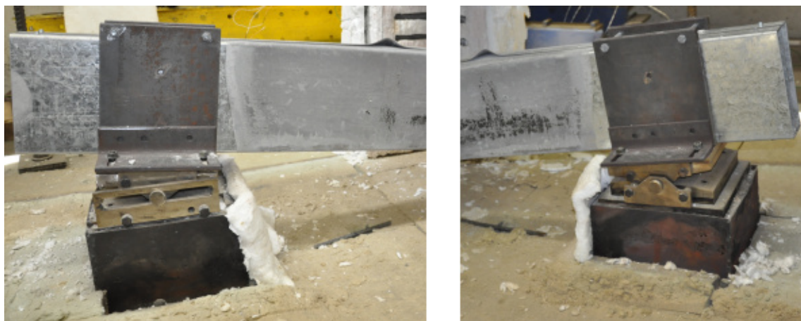
Figure F.43 – Front views of the failure mode of the specimen B-2R_3
