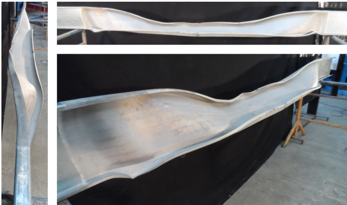
Figure 3.38 – Failure modes of the test beam B_ka+kr-C_3 under fire conditions
