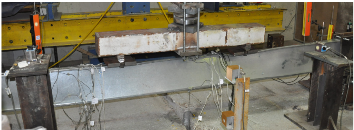
Figure B.12 – Front view of the failure mode of specimen B-I_2
