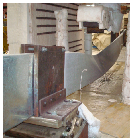
Figure F.7 – Lateral views of the failure mode of the specimen B-C_2
