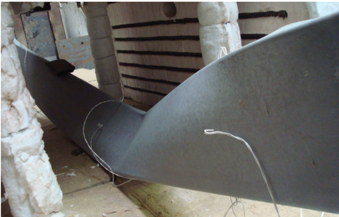
Figure F.4 – Detail view of the failure mode of the specimen B-C_1
