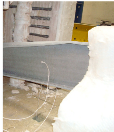
Figure F.5 – Front views of the failure mode of the specimen B-C_2
