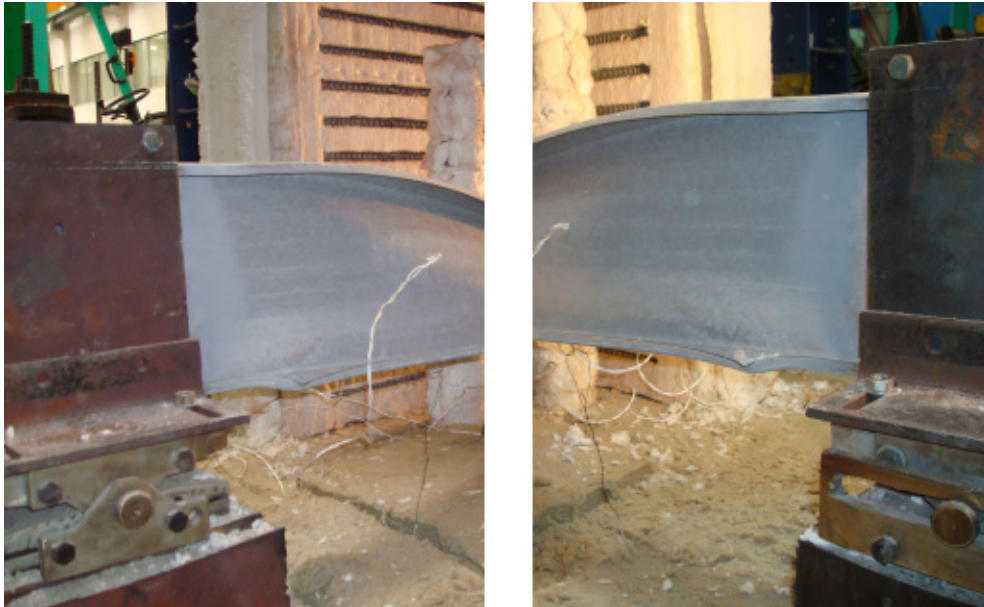
Figure F.87 – Front views of the failure mode of the specimen B_ka+kr-I_2
