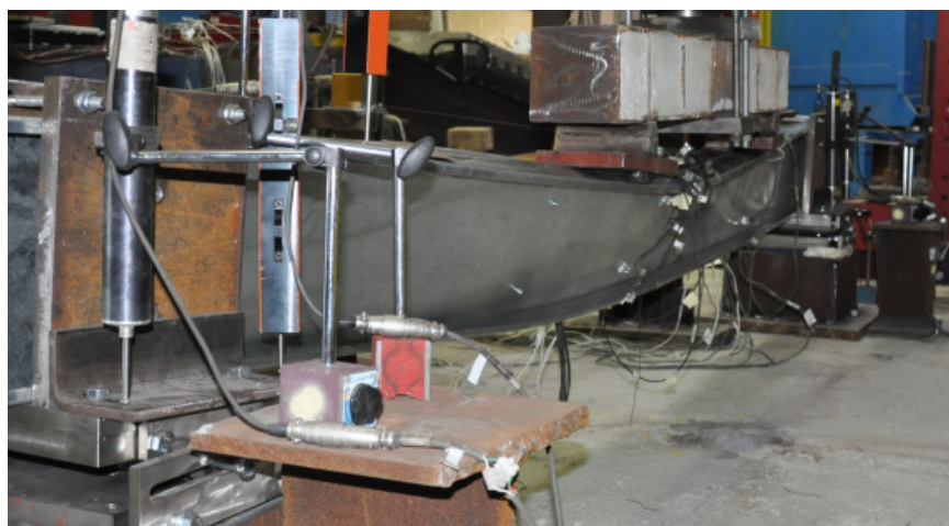
Figure B.13 – Back view of the failure mode of specimen B-I_2
