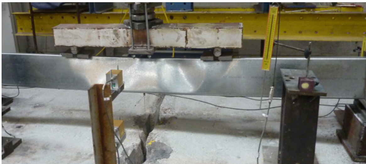
Figure B.18 – Front view of the failure mode of specimen B-R_1
