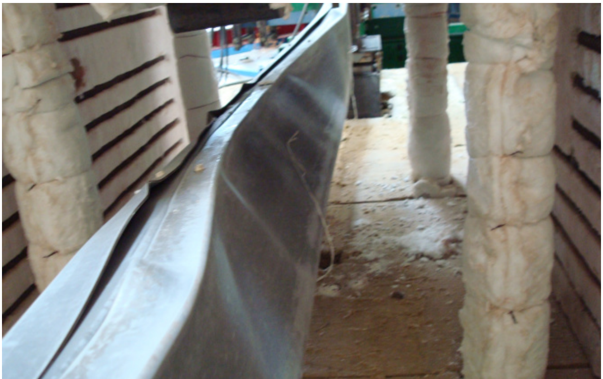
Figure F.71 – Detail view of the failure mode of the specimen B_ka-2R_1
