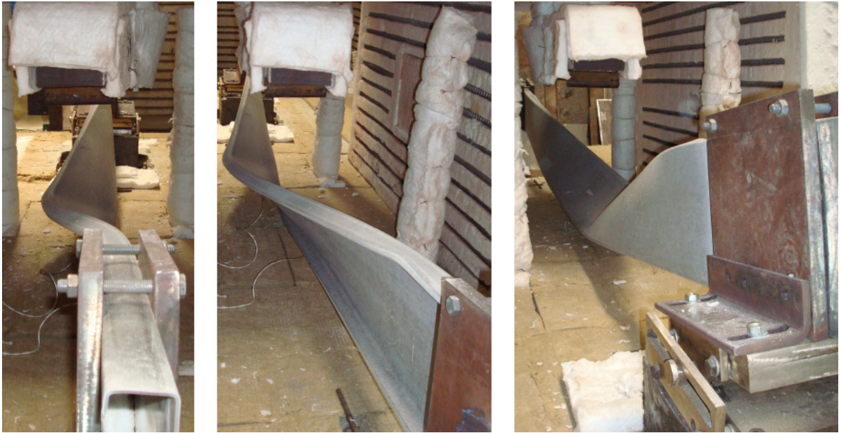
Figure F.11 – Lateral views of the failure mode of the specimen B-C_3
