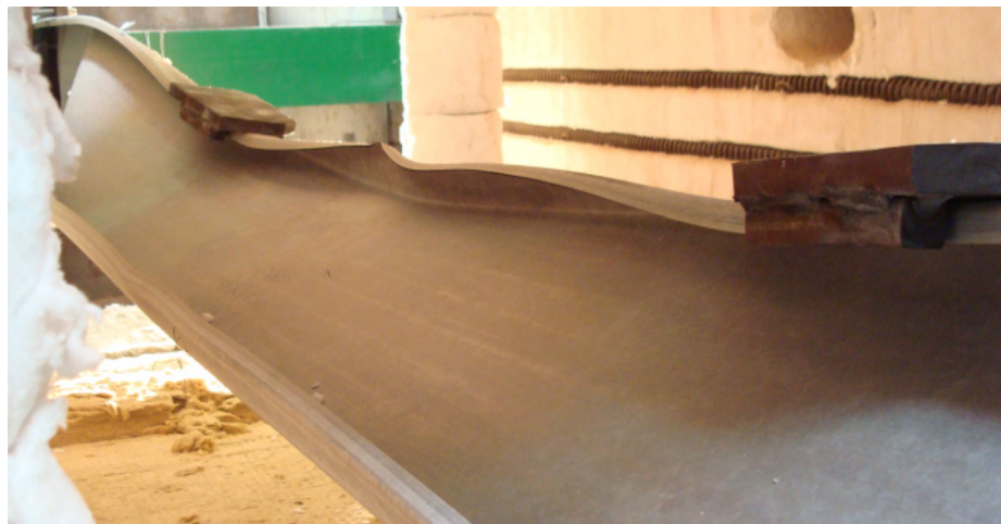
Figure F.81 – Detail view of the failure mode of the specimen B_ka+kr-C_2
