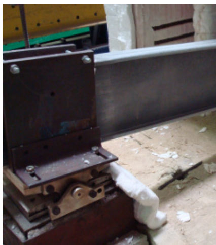
Figure F.18 – Back views of the failure mode of the specimen B-I_2
