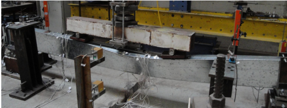
Figure B.31 – Back view of the failure mode of specimen B-2R_2
