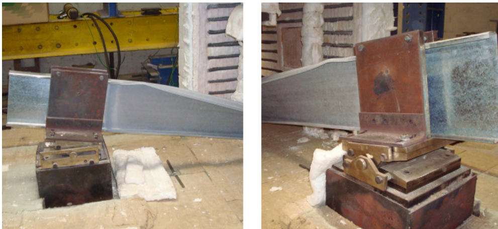
Figure F.9 – Front views of the failure mode of the specimen B-C_3
