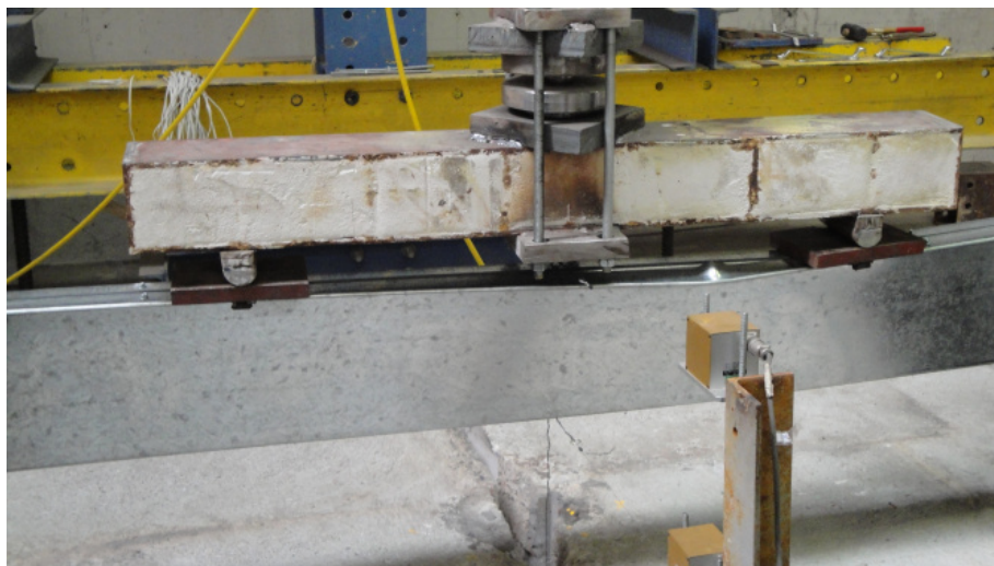
Figure 3.33 – Failure modes of the test beam B-2R_1 at ambient temperature
