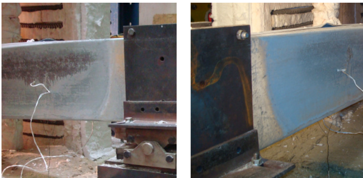
Figure F.95 – Front views of the failure mode of the specimen B_ka+kr-2R_1
