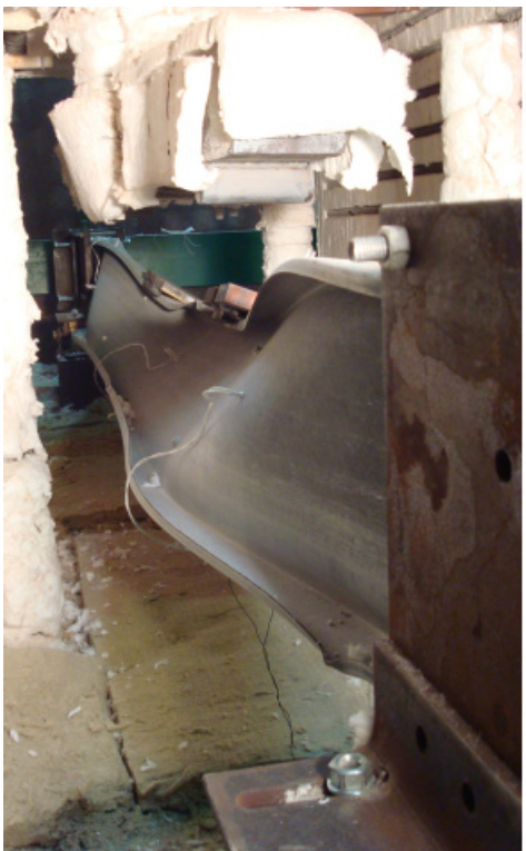
Figure F.86 – Lateral views of the failure mode of the specimen B_ka+kr-I_1
