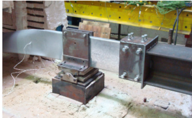
Figure F.51 – Back views of the failure mode of the specimen B_ka-C_2
