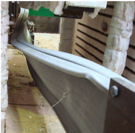
Figure F.58 – Lateral views of the failure mode of the specimen B_ka-I_1
