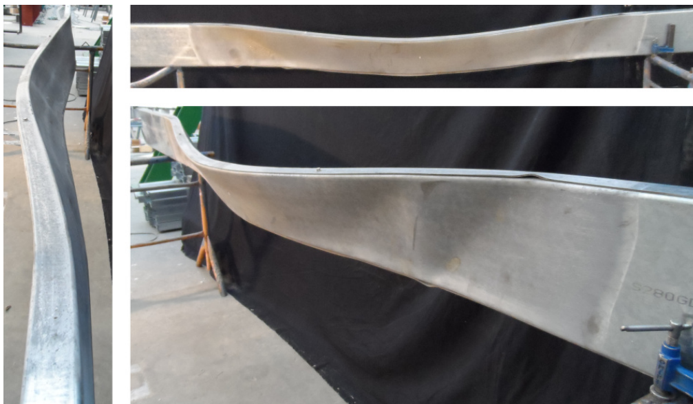
Figure 3.40 – Failure modes of the test beam B_ka+kr-R_2 under fire conditions
