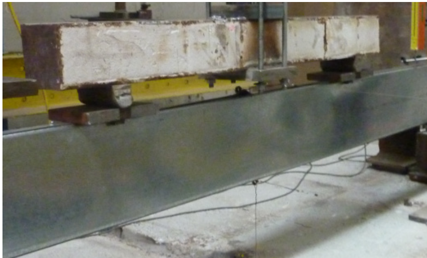
Figure B.20 – Detail view of the failure mode of specimen B-R_1
