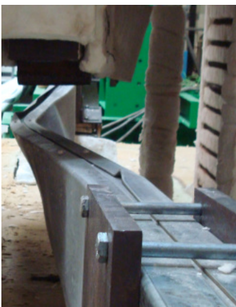
Figure F.37 – Lateral views of the failure mode of the specimen B-2R_1
