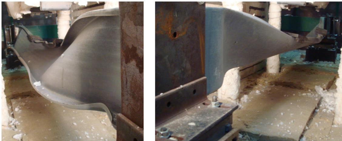
Figure F.83 – Lateral views of the failure mode of the specimen B_ka+kr-C_3
