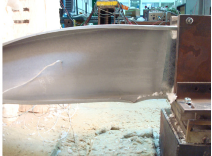
Figure F.85 – Front views of the failure mode of the specimen B_ka+kr-I_1
