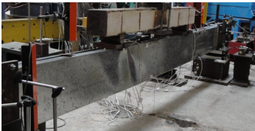
Figure B.30 – Front view of the failure mode of specimen B-2R_2
