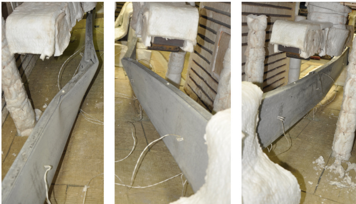
Figure F.29 – Lateral views of the failure mode of the specimen B-R_2
