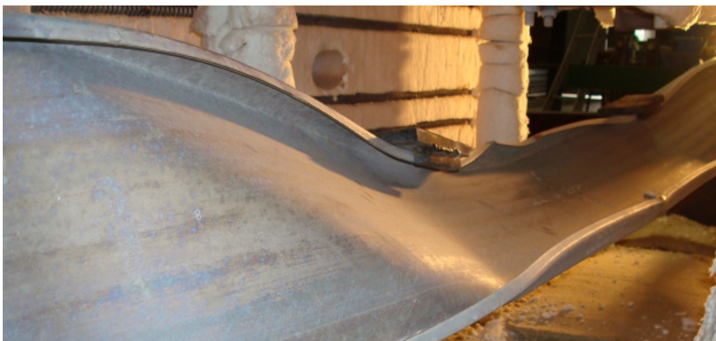
Figure F.84 – Detail view of the failure mode of the specimen B_ka+kr-C_3
