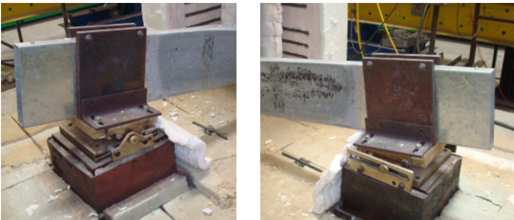
Figure F.32 – Back views of the failure mode of the specimen B-R_3
