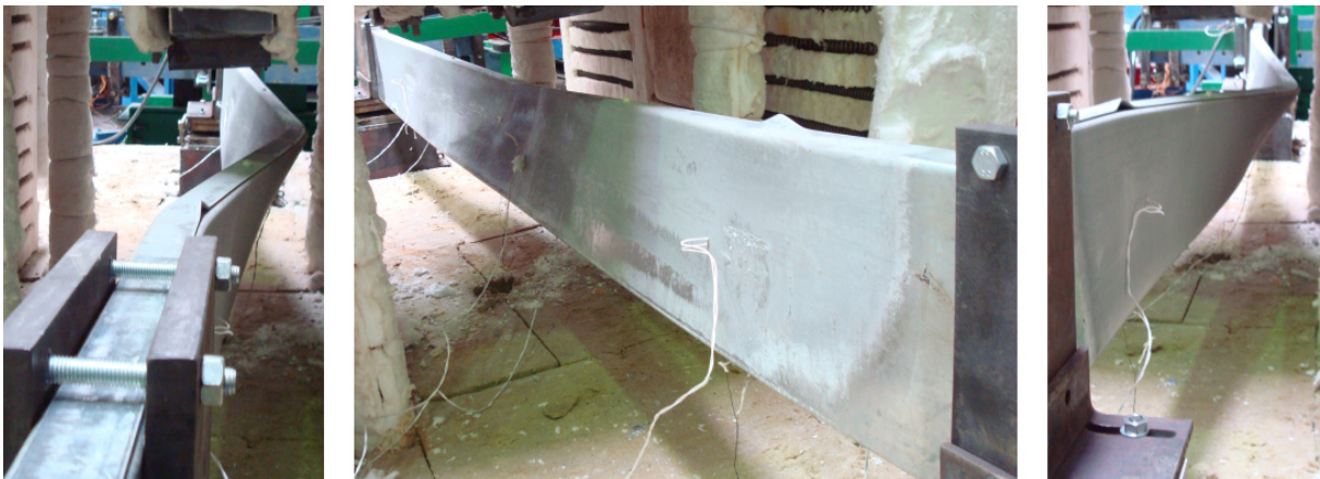
Figure F.65 – Lateral views of the failure mode of the specimen B_ka-R_1
