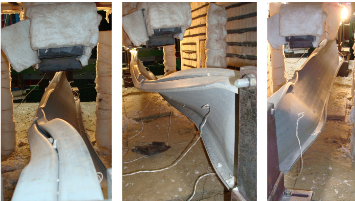
Figure F.88 – Lateral views of the failure mode of the specimen B_ka+kr-I_2
