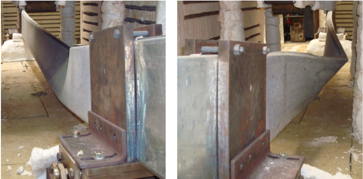
Figure F.33 – Lateral views of the failure mode of the specimen B-R_3
