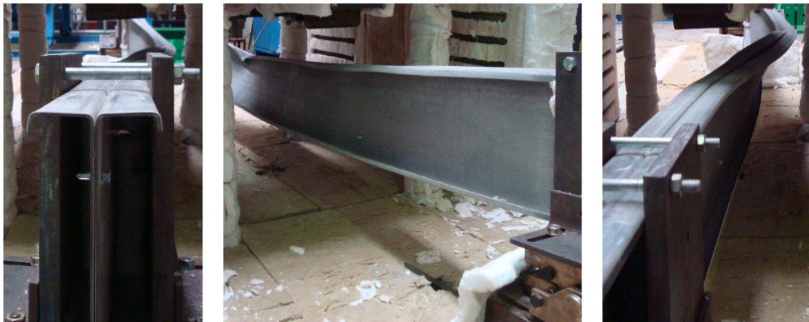
Figure F.19 – Lateral views of the failure mode of the specimen B-I_2
