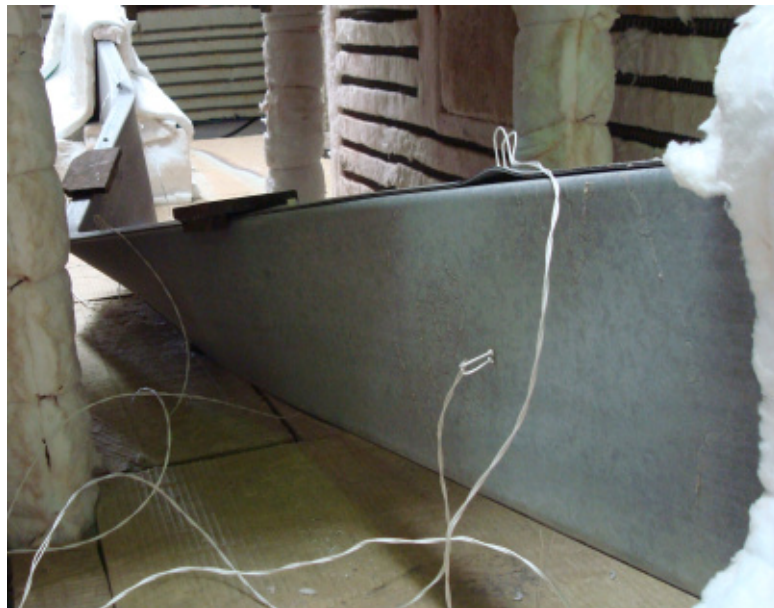
Figure F.28 – Detail view of the failure mode of the specimen B-R_1
