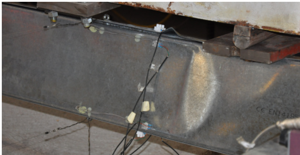
Figure B.23 – Detail view of the failure mode of specimen B-R_2
