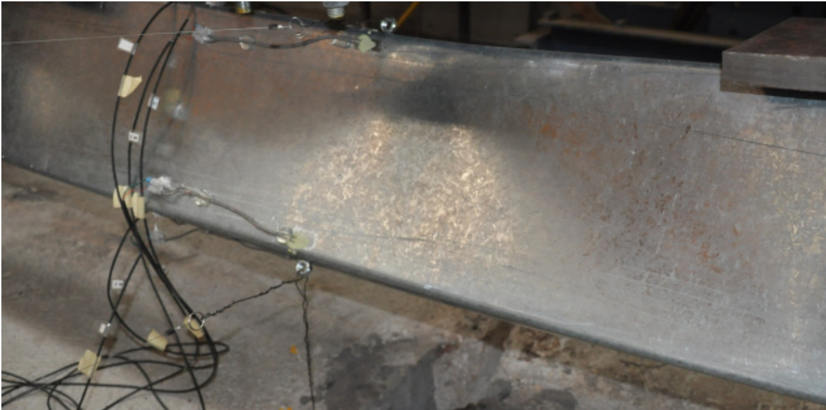
Figure B.9 – Detail view of the failure mode of specimen B-C_3
