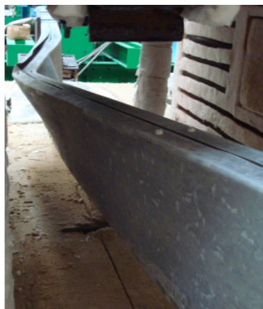
Figure F.37 – Lateral views of the failure mode of the specimen B-2R_1
