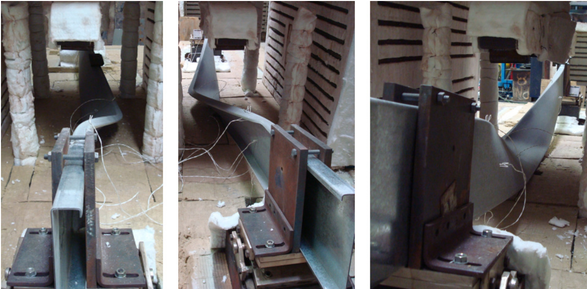
Figure F.3 – Lateral views of the failure mode of the specimen B-C_1
