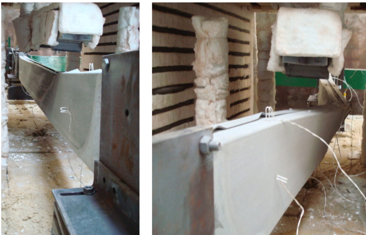
Figure F.75 – Lateral views of the failure mode of the specimen B_ka-2R_3
