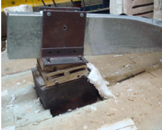
Figure F.35 – Front views of the failure mode of the specimen B-2R_1
