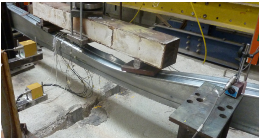
Figure B.16 – Back view of the failure mode of specimen B-I_3
