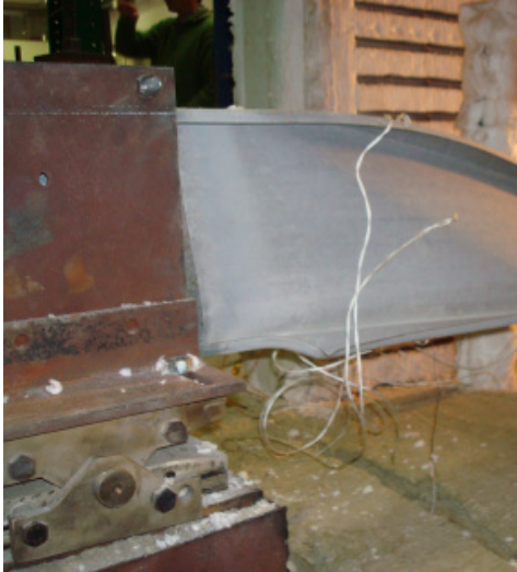
Figure F.85 – Front views of the failure mode of the specimen B_ka+kr-I_1
