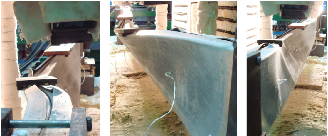
Figure F.99 – Lateral views of the failure mode of the specimen B_ka+kr-2R_2
