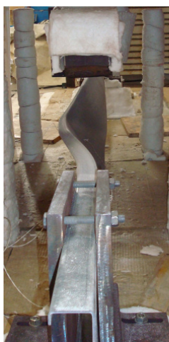
Figure F.7 – Lateral views of the failure mode of the specimen B-C_2
