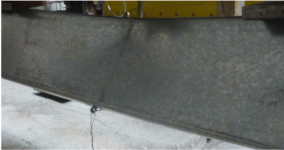
Figure B.3 – Detail view of the failure mode of specimen B-C_1
