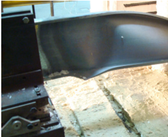
Figure F.79 – Front views of the failure mode of the specimen B_ka+kr-C_2
