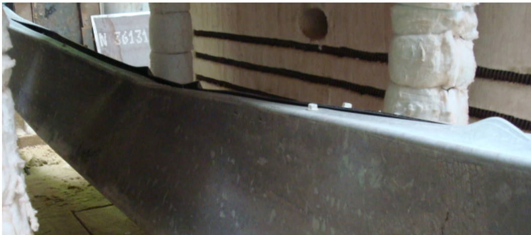
Figure F.42 – Detail view of the failure mode of the specimen B-2R_2
