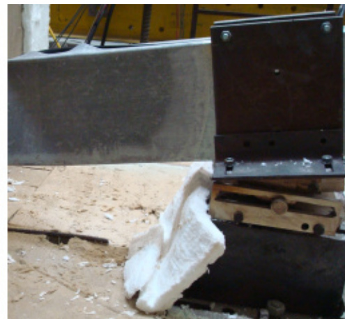
Figure F.36 – Back views of the failure mode of the specimen B-2R_1
