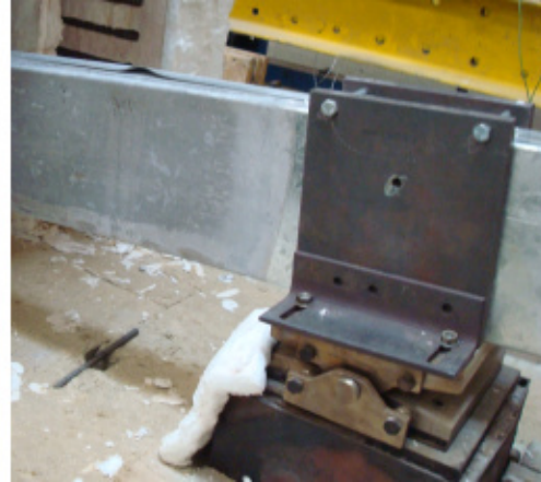
Figure F.35 – Front views of the failure mode of the specimen B-2R_1
