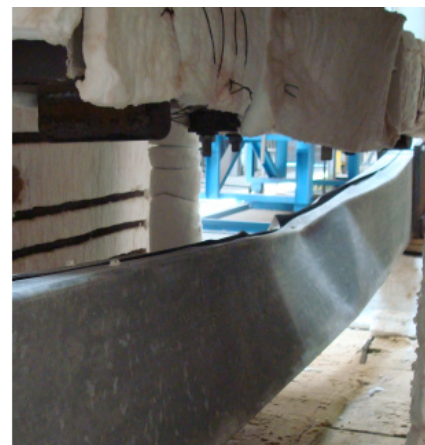
Figure F.37 – Lateral views of the failure mode of the specimen B-2R_1
