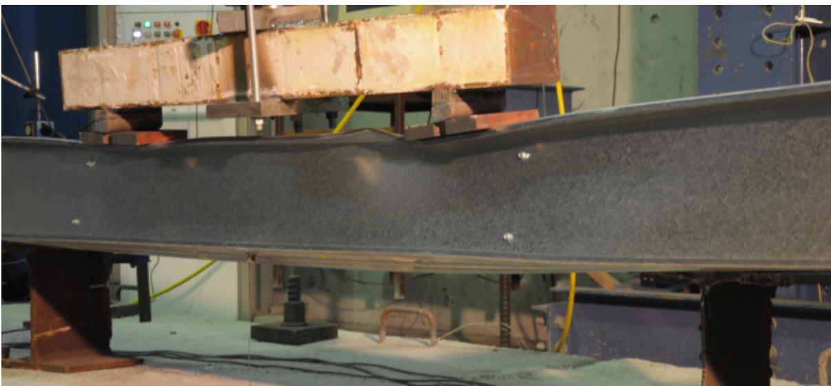
Figure B.10 – Front view of the failure mode of specimen B-I_1
