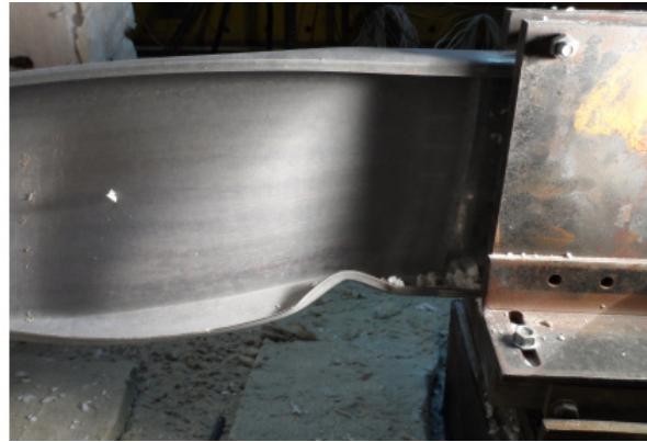
Figure F.76 – Front views of the failure mode of the specimen B_ka+kr-C_1
