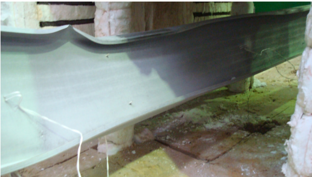
Figure F.63 – Detail view of the failure mode of the specimen B_ka-I_3
