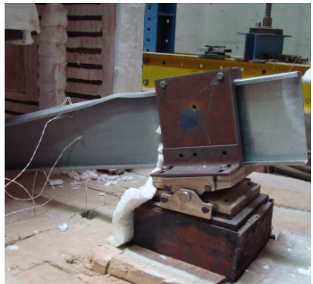
Figure F.1 – Front views of the failure mode of the specimen B-C_1
