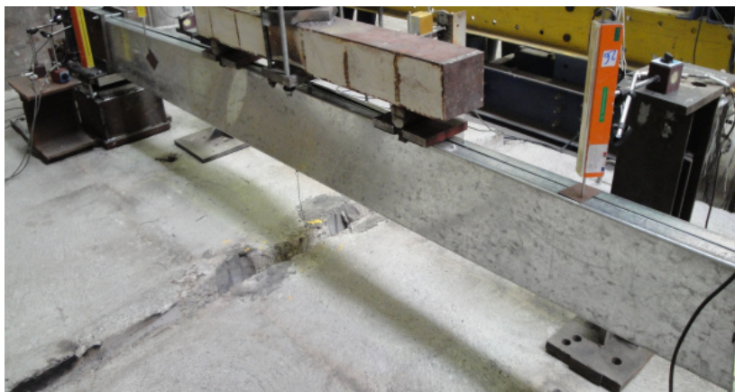
Figure B.27 – Front view of the failure mode of specimen B-2R_1
