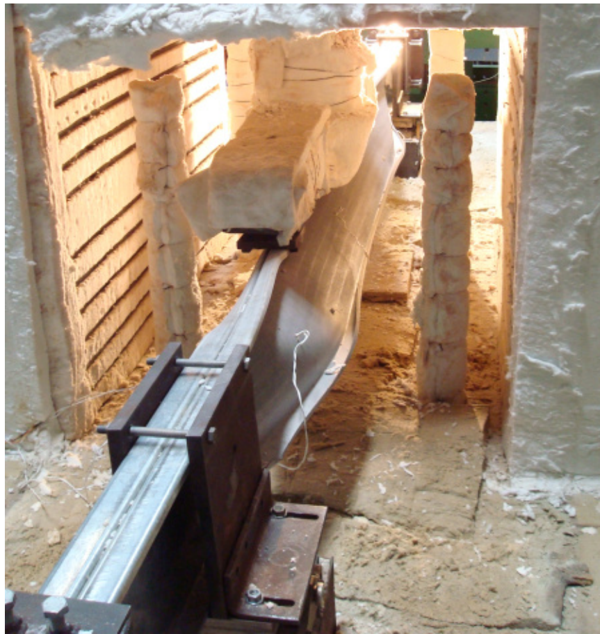
Figure F.89 – Detail view of the failure mode of the specimen B_ka+kr-I_2
