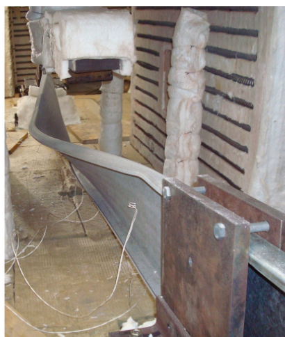
Figure F.7 – Lateral views of the failure mode of the specimen B-C_2
