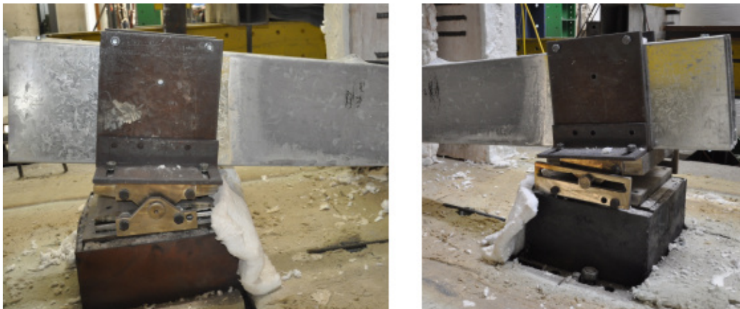
Figure F.44 – Back views of the failure mode of the specimen B-2R_3
