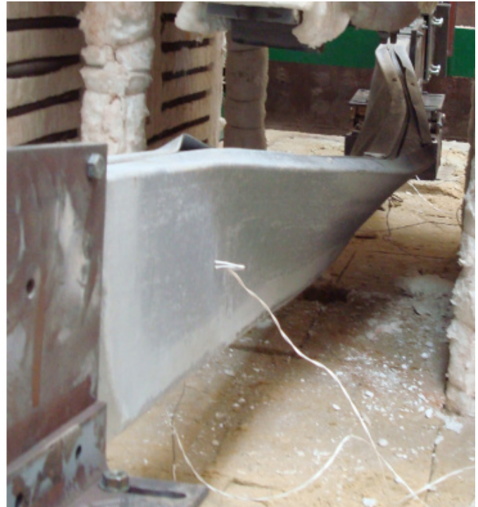
Figure F.70 – Lateral views of the failure mode of the specimen B_ka-2R_1
