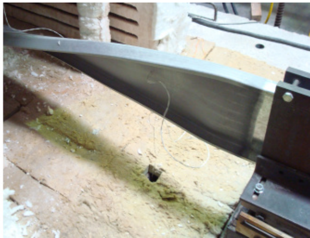
Figure F.52 – Front views of the failure mode of the specimen B_ka-C_2
