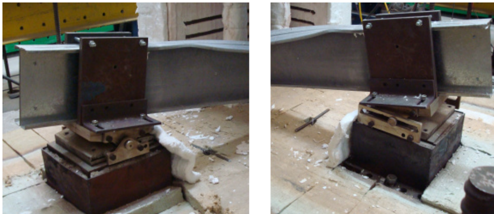
Figure F.14 – Back views of the failure mode of the specimen B-I_1
