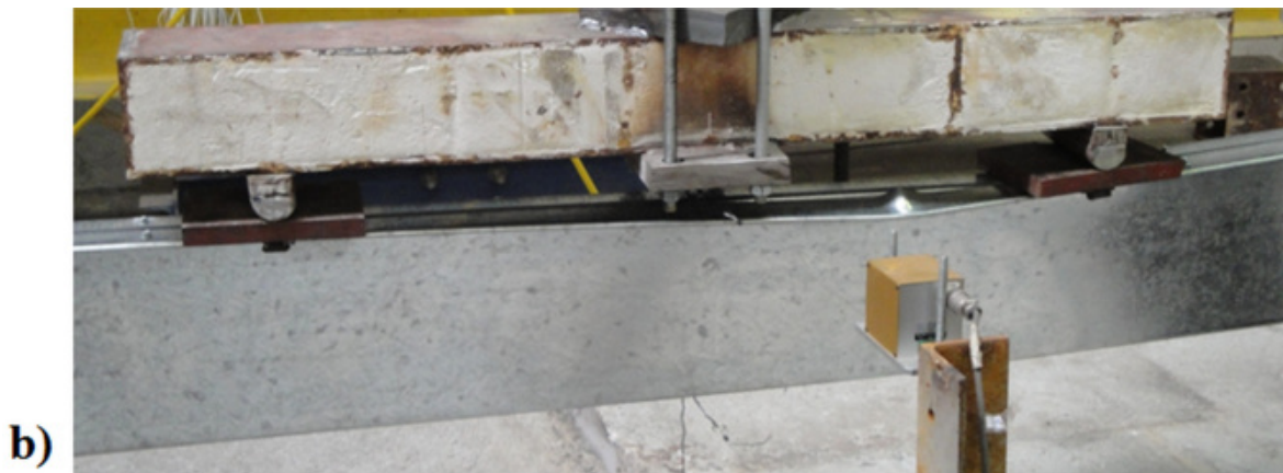
Figure 4.21 – Numerical (a) and experimental (b) failure modes for the 2R beam
