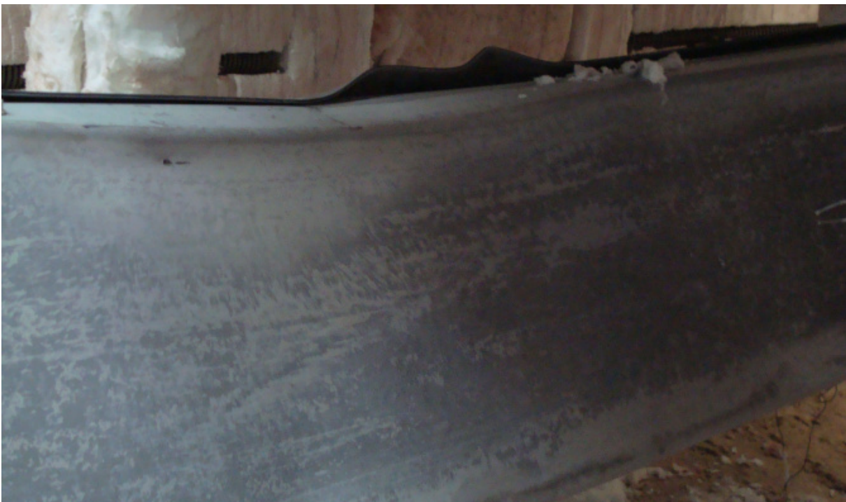
Figure F.73 – Detail view of the failure mode of the specimen B_ka-2R_2
