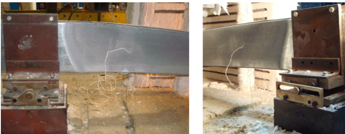
Figure F.93 – Front views of the failure mode of the specimen B_ka+kr-R_3
