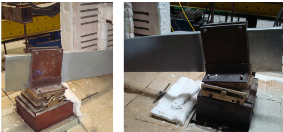
Figure F.10 – Back views of the failure mode of the specimen B-C_3
