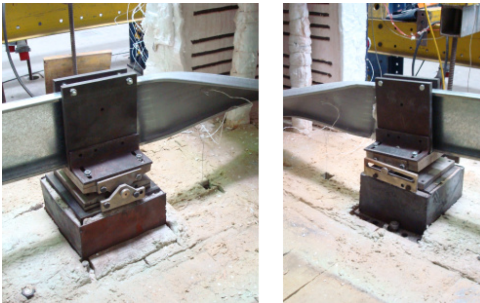
Figure F.48 – Front views of the failure mode of the specimen B_ka-C_1
