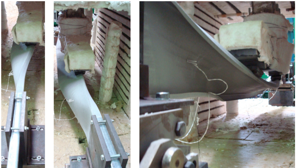
Figure F.49 – Lateral views of the failure mode of the specimen B_ka-C_1
