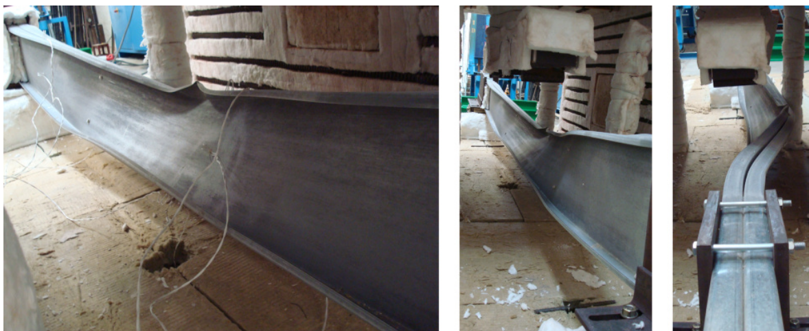
Figure 3.35 – Failure modes of the test beam B-I_1 under fire conditions
