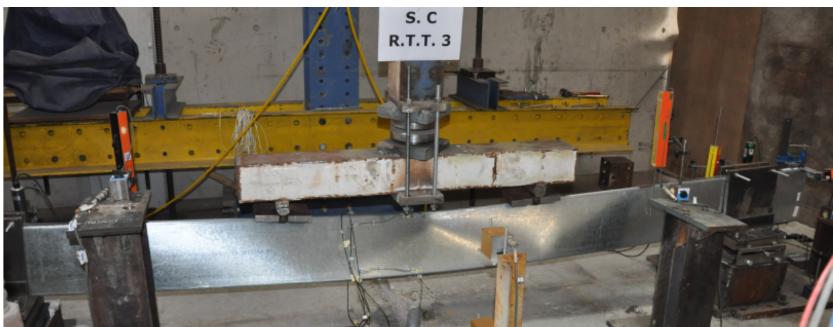
Figure B.8 – Back view of the failure mode of specimen B-C_3
