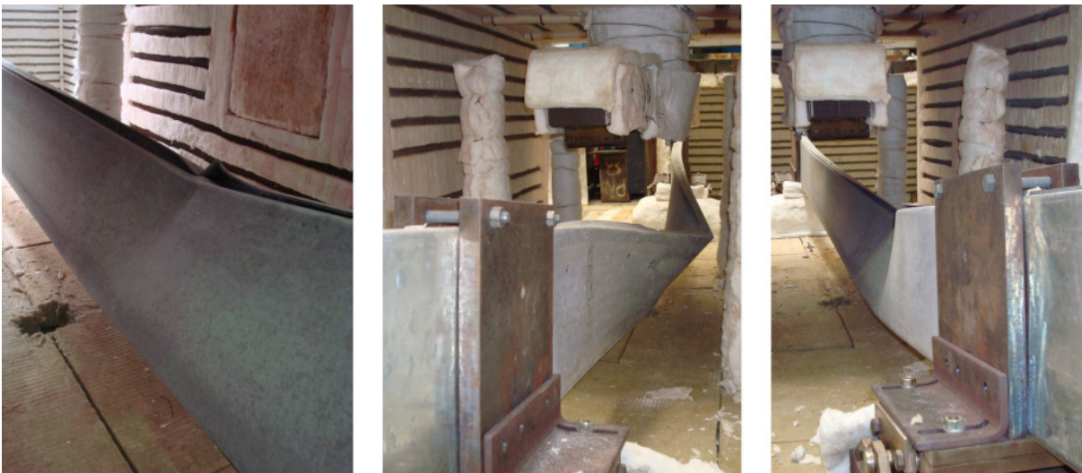
Figure 3.36 – Failure modes of the test beam B-R_3 under fire conditions
