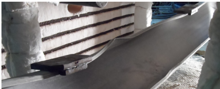
Figure F.78 – Detail view of the failure mode of the specimen B_ka+kr-C_1
