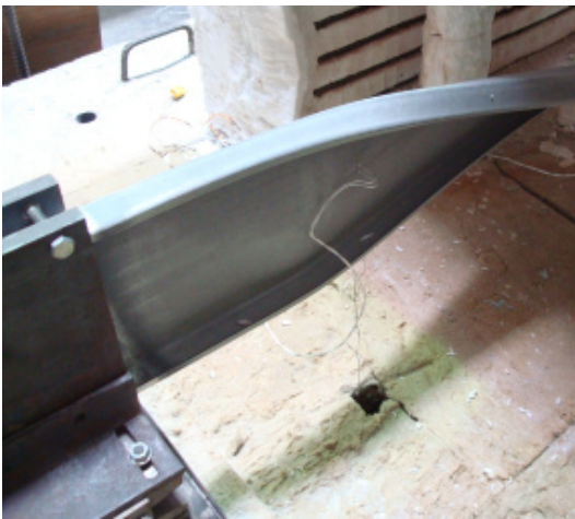
Figure F.52 – Front views of the failure mode of the specimen B_ka-C_2
