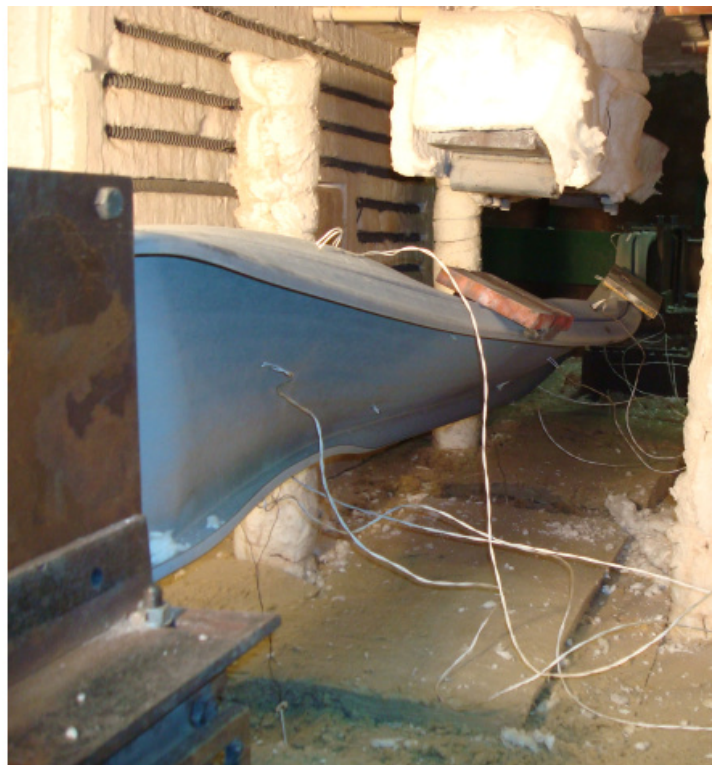
Figure F.86 – Lateral views of the failure mode of the specimen B_ka+kr-I_1
