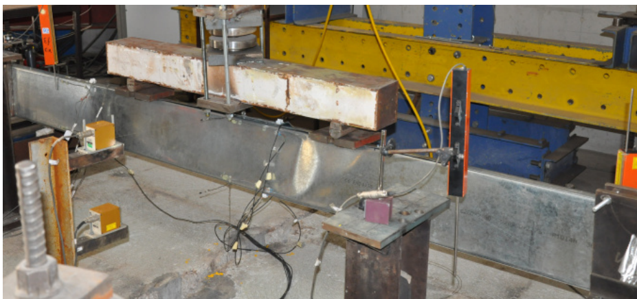
Figure B.21 – Front view of the failure mode of specimen B-R_2
