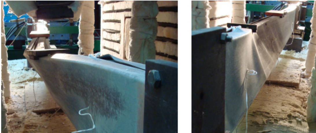
Figure F.96 – Lateral views of the failure mode of the specimen B_ka+kr-2R_1
