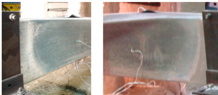
Figure F.101 – Front views of the failure mode of the specimen B_ka+kr-2R_3
