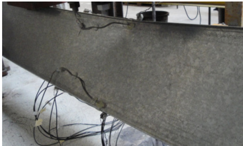
Figure B.6 – Detail view of the failure mode of specimen B-C_2
