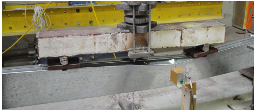
Figure B.28 – Back view of the failure mode of specimen B-2R_1
