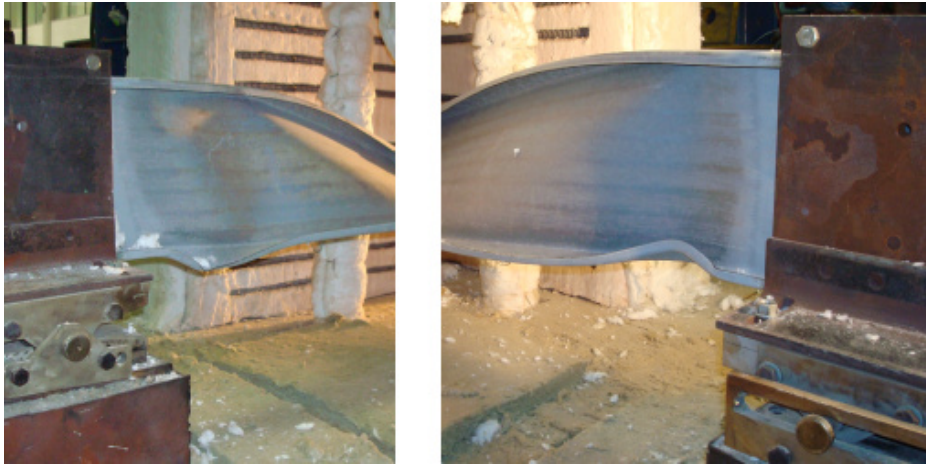
Figure F.82 – Front views of the failure mode of the specimen B_ka+kr-C_3
