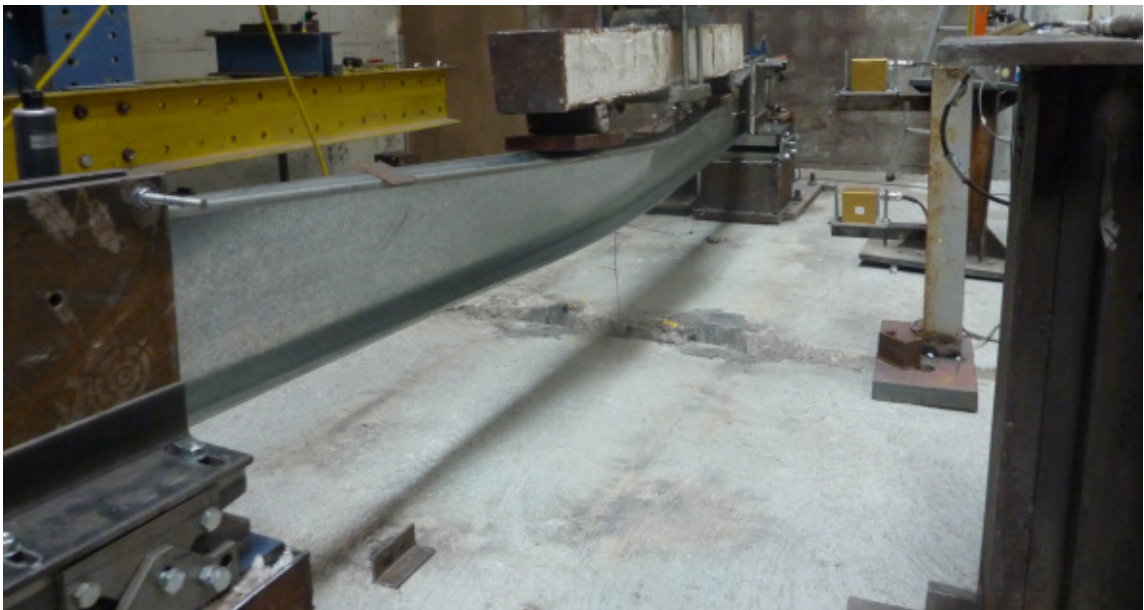
Figure B.1 – Front view of the failure mode of specimen B-C_1
