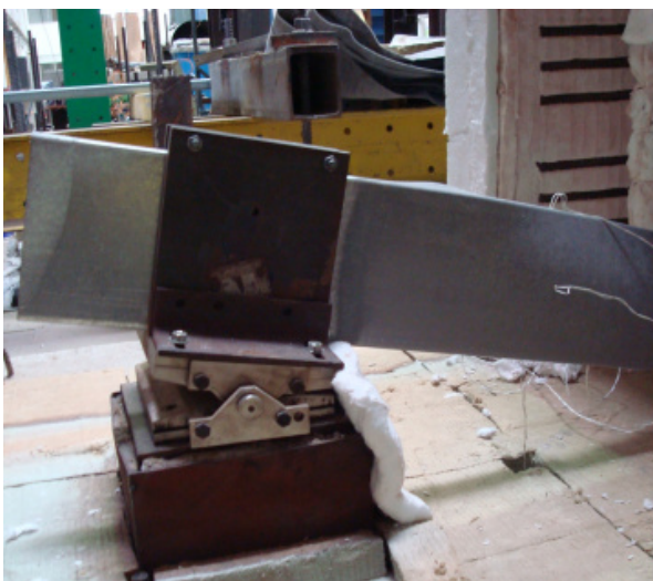
Figure F.2 – Back views of the failure mode of the specimen B-C_1
