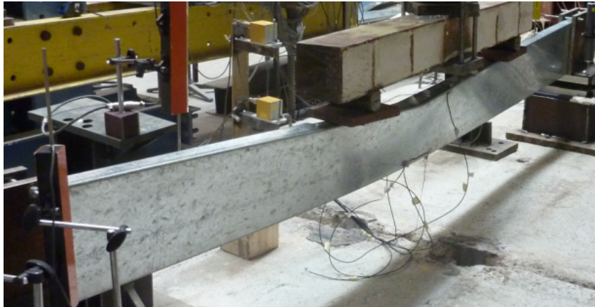
Figure B.25 – Back view of the failure mode of specimen B-R_3
