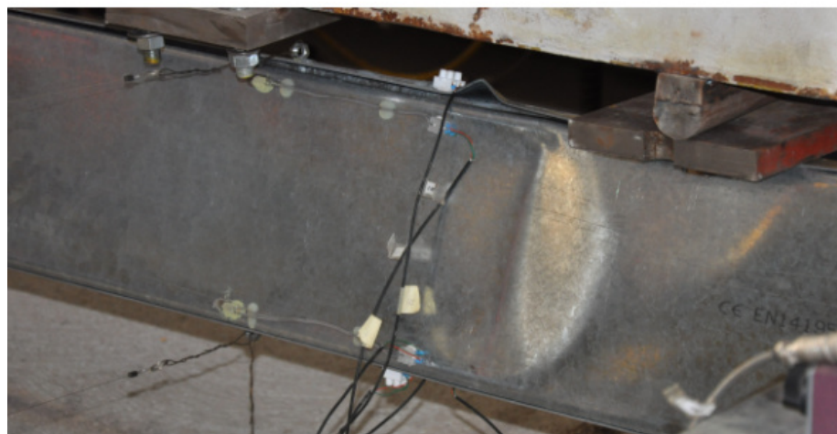
Figure 3.32 – Failure modes of the test beam B-R_2 at ambient temperature
