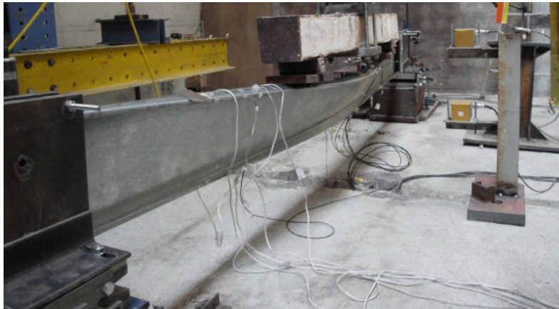
Figure B.4 – Front view of the failure mode of specimen B-C_2
