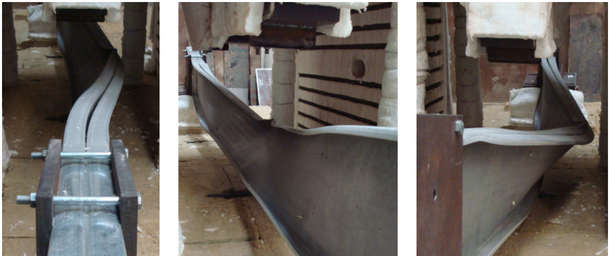
Figure F.23 – Lateral views of the failure mode of the specimen B-I_3
