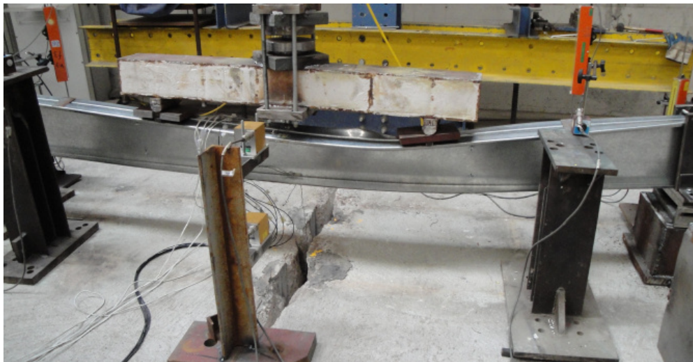
Figure 3.31 – Failure modes of the test beam B-I_3 at ambient temperature
