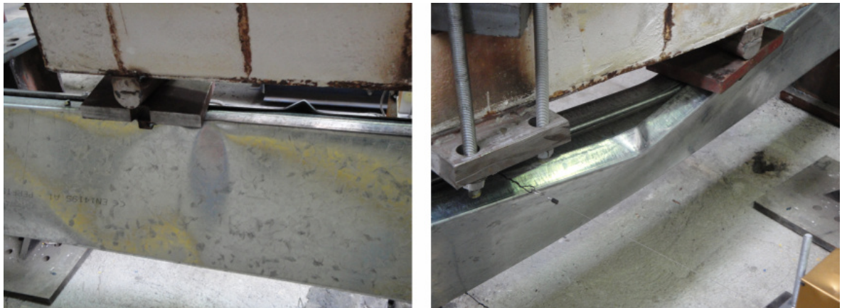
Figure B.29 – Detail views of the failure mode of specimen B-2R_1
