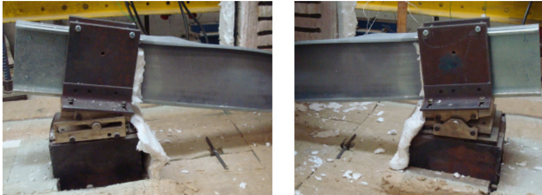
Figure F.13 – Front views of the failure mode of the specimen B-I_1
