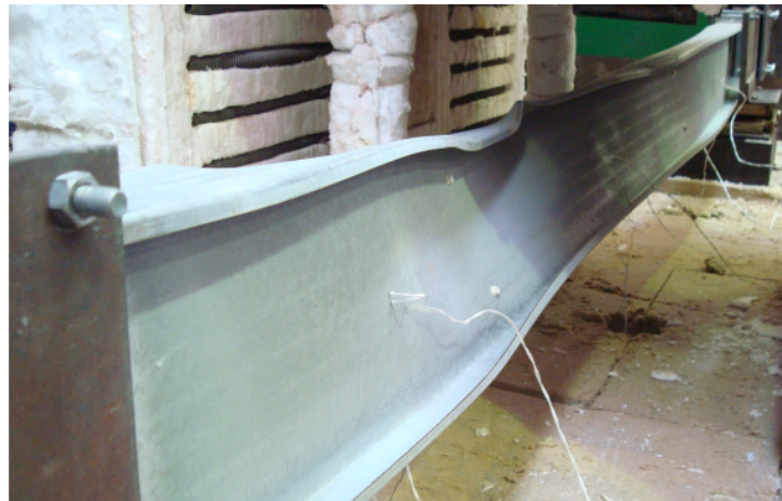
Figure F.58 – Lateral views of the failure mode of the specimen B_ka-I_1
