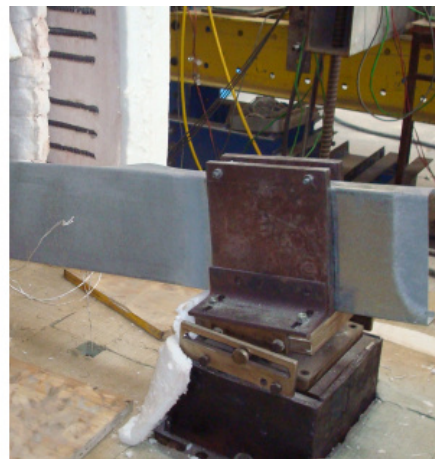
Figure F.6 – Back views of the failure mode of the specimen B-C_2
