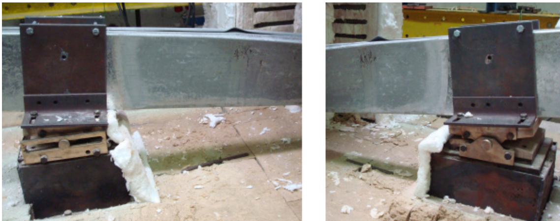
Figure F.39 – Front views of the failure mode of the specimen B-2R_2
