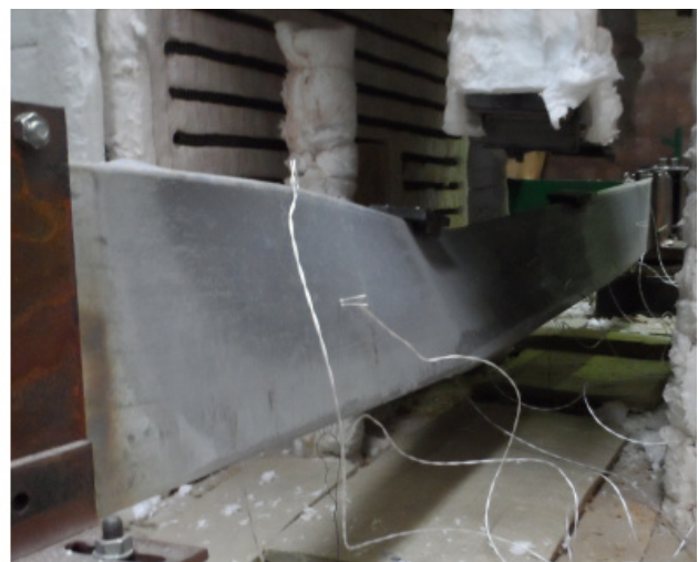
Figure F.90 – Lateral views of the failure mode of the specimen B_ka+kr-R_1
