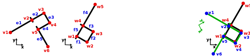
Figure 2.12: Two maps with different coordinate systems (left). The result of merging maps (right).
