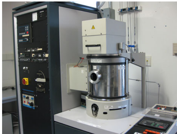
Figura 5: Edwards Coating System E306A [32].
