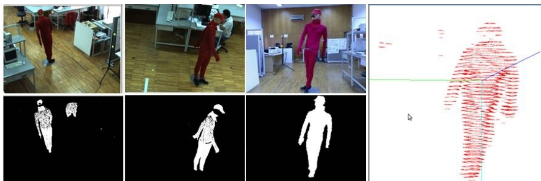
Figure 4.19: Result of 3D reconstruction when a mobile sensor is augmented to the network (corresponding to Fig. 4.18 ); In order to have more details of the scene, a mobile sensor is navigated close to the mannequin and its view is integrated as a new node in the network. The left two columns are the images corresponding to the two fixed cameras and the third column from left is the image corresponding to the mobile camera. The results of the 3D reconstruction by using two fixed IS-camera couples and a new augmented couple is demonstrated in the right column.
