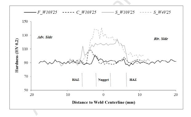
Figure 8 - Hardness distribution in the cross section of the F\_W10V25, C\_W10V25, S\_W10V25 and S\_W4V25 welds.
