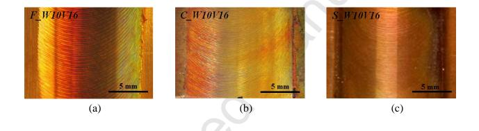
Figure 2 - Surface appearance of the F\_W10V16 (a), C\_W10V16 (b) and S\_W10V16 (c) welds.
