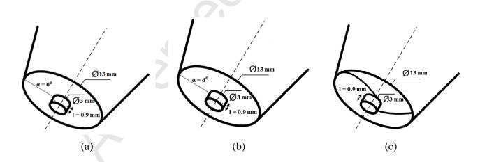
Figure 1 - Schematic representation of the flat (a) conical concave (b) and scrolled (c) shouldered tools.
