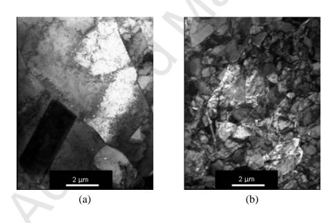
Figure 7 - TEM micrographs illustrating the grain structure in the nugget of the C\_W10V16 (a) and S\_W10V16 (b) welds.
