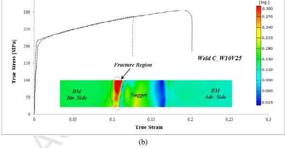
Figure 9 - Local stress-strain curves corresponding to different zones (BM and Nugget) of transverse specimens taken from the welds S\_W10V25 (a) and C\_W10V25 (b), and images of the longitudinal strain distribution in the specimens just after maximum load.
