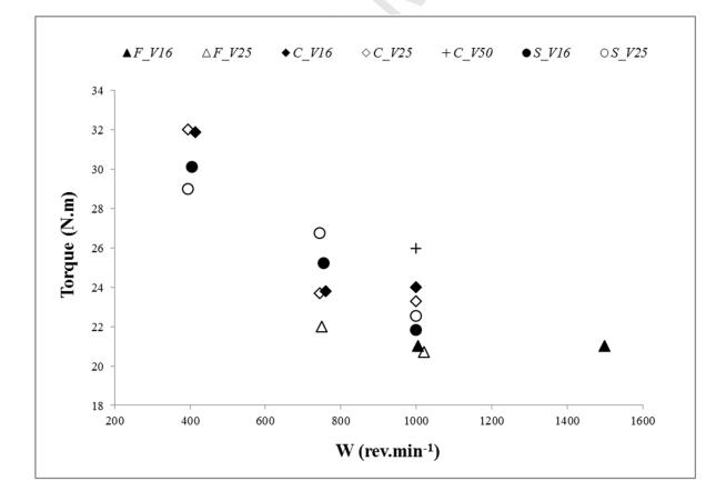
Figure 5 - Influence of rotational speed and tool geometry on average welding Torque.
