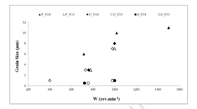
Figure 6 - Influence of rotational speed and tool geometry on the weld nugget average grain size.
