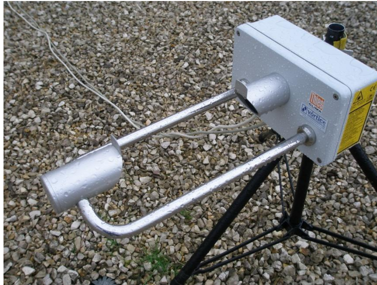
Figure 2.3 Example of disdrometer (Thies Clima) available in the Laboratory of Hydraulics, Water Resources and Environment of the Civil Engineering Department of the Faculty of Sciences and Technology, University of Coimbra.
