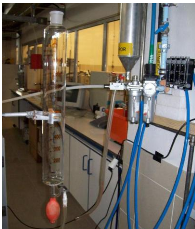
Figure 5.2 - Feed air flow measuring.
