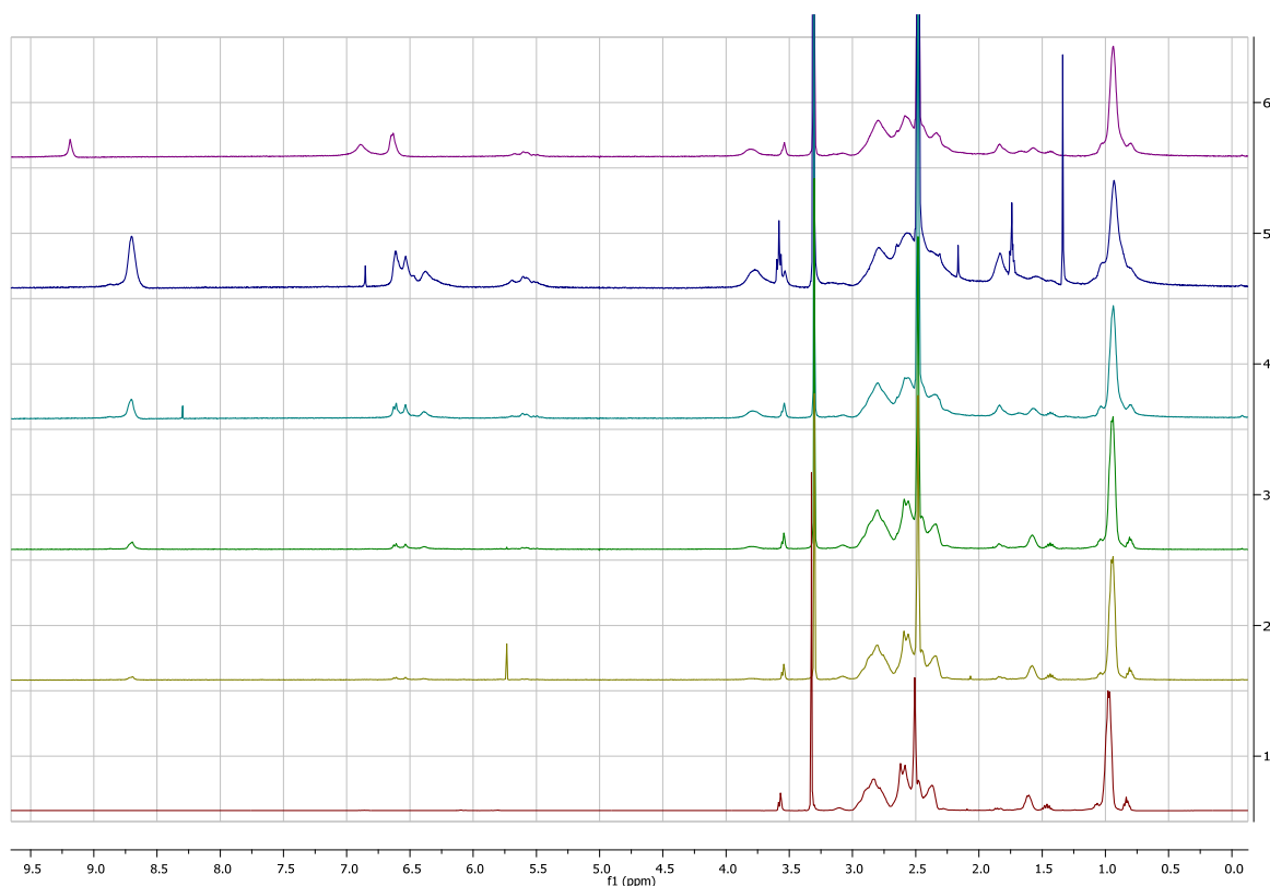
Figure 4.12: ^1\text{H-NMR} spectra of PK30 (bottom, 1), of dopamine-modified PK30 at 5% (2), 10% (3), 25 (4) and 50% (5) aimed conversion using TEA and of tyramine modified PK30 at 25% aimed conversion (6, top) in DMSO.
