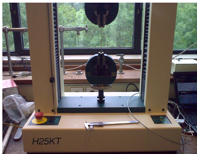
Figure 4.24: Adhesive testing set-up with aluminium adherends in lap shear configuration
