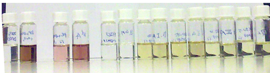
Figure 4.22: Photograph of UV-Vis samples before and after NaIO 4 oxidation. From left to right: dopamine-HCl, dopamine-pyrrolic model compound, PK 30 , PK 30-5 , PK 30-10 , PK 30-25 and PK 30-50
