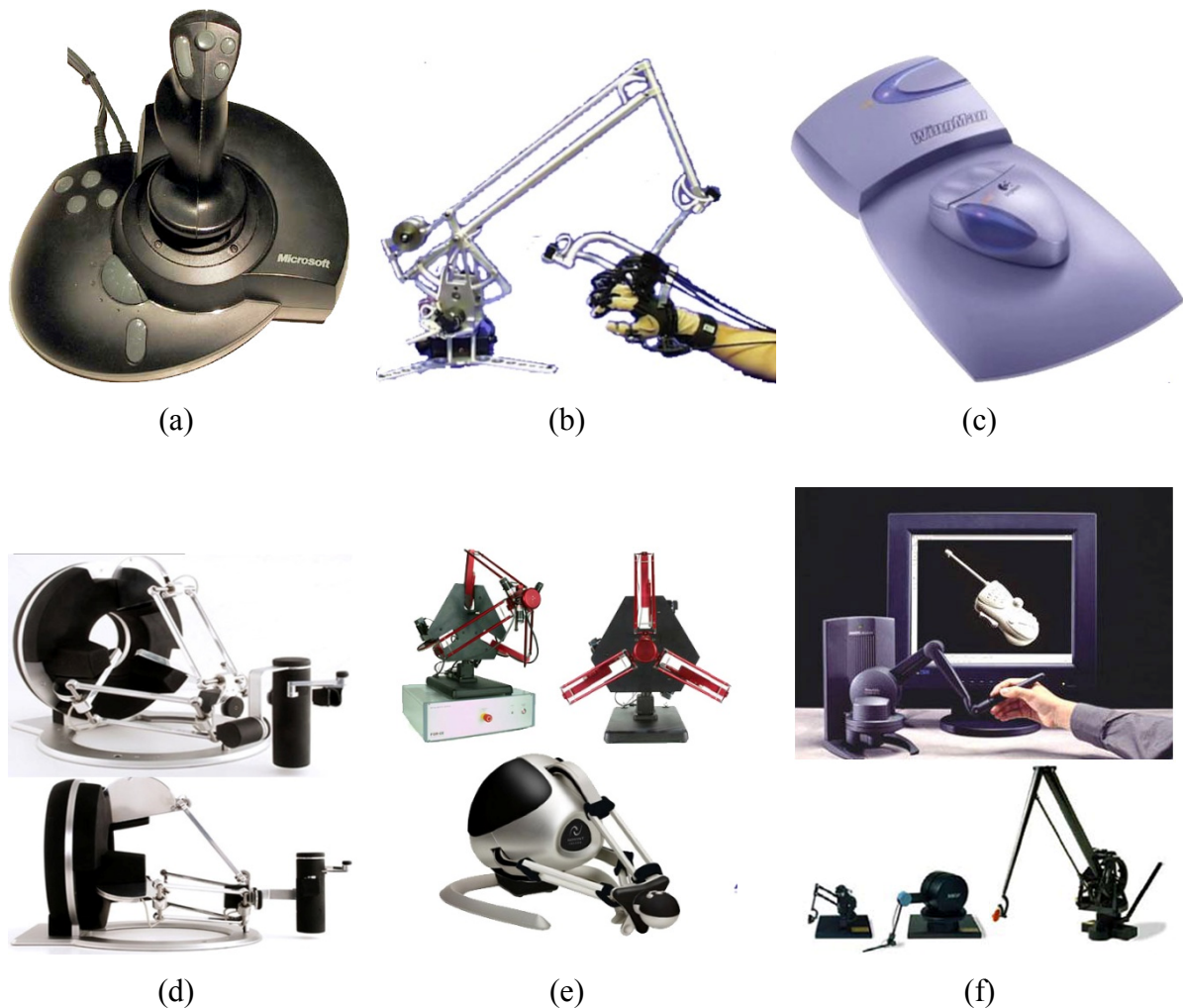
Figure 2 – Haptic devices. (a) SideWinder Joystick; (b) DataGlove Cyberglove; (c) WingMan Mice; (d) Omega.7 from Force Dimension; (e) Delta Haptic devices (Force Dimension Delta and Novint Falcon); (f) Phantom from SensAble.
