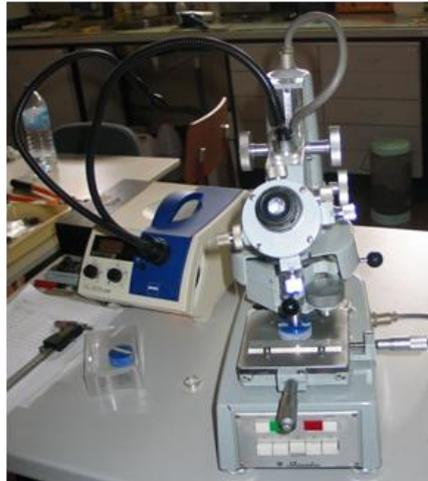
Figura 5 - Shimadzu Microhardness Tester
