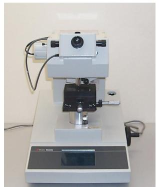
Fig. 3.4: Struers hardness testing equipment, model Duramin used to perform Vickers microhardness tests.
