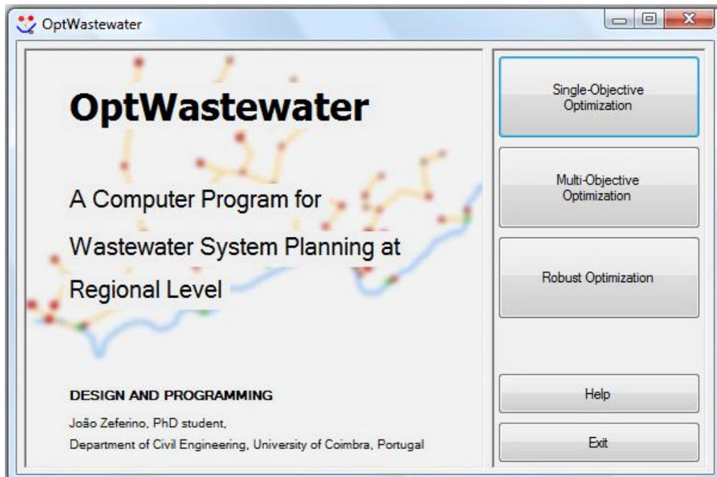
Figure 8.3 - OptWastewater Entrance Window
