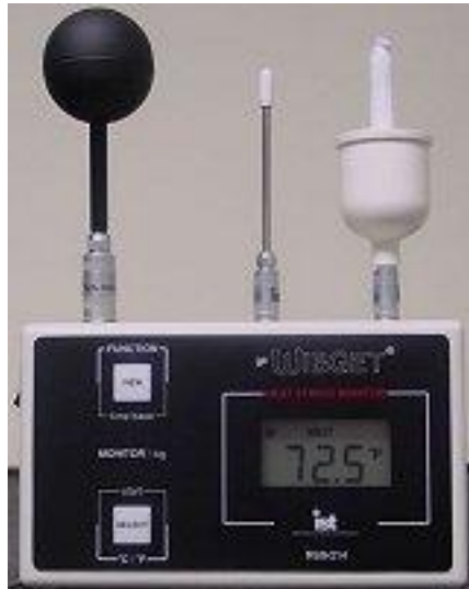
Figure 5 - Equipment to assess WBGT index (Ross and Barker, 2005).
