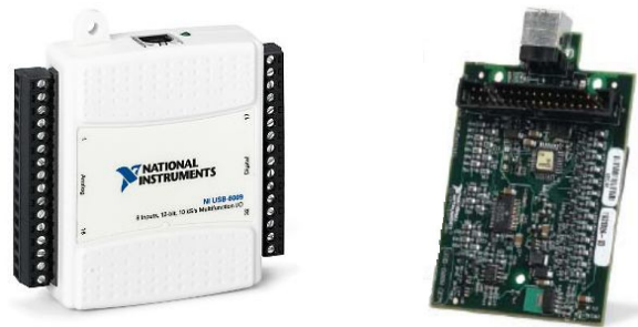
Figure 20 - DAQ Module NI 6009; normal view (a) and internal view (b) of the device; [52]
