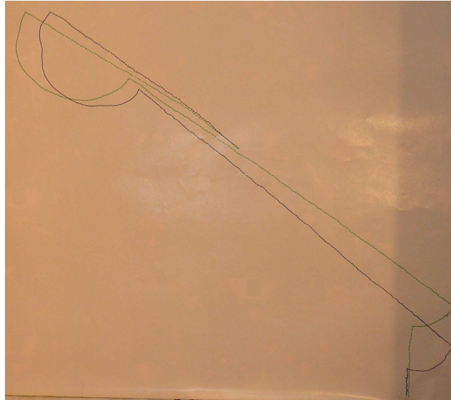
Figure 8.11: Paths of the robot forward (black line) and backwards (green line), in the arithmetic mode and data distribution to at least three locations.
