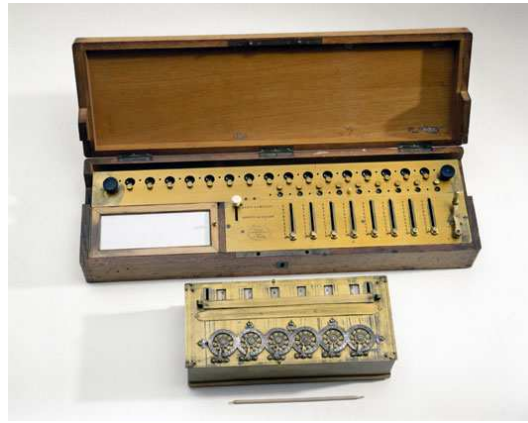
Figure 1.1: Picture of a replica of the first commercial calculator, which is in exhibition at the Science Museum in London 4 .
