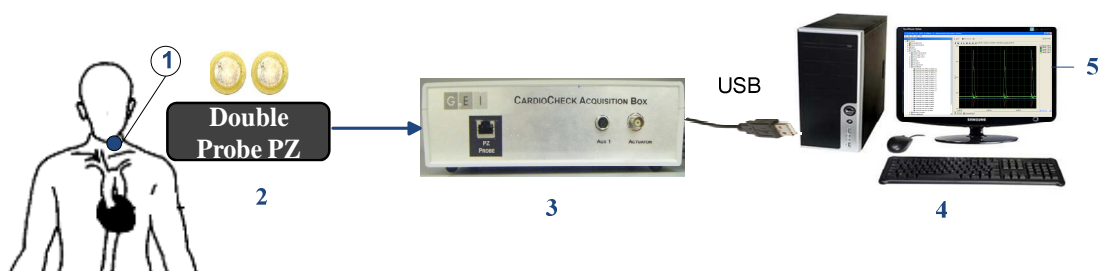
Figure 3.1- Acquisition system scheme. 1- Common carotid artery, 2- Measurement probe (Double PZ probe), 3- Data acquisition system ( CardioCheck Acquisition Box), 4- Data logging processing and storage (PC), 5- NI software ( Measurement & Automation ) or Cardio-Check database.
