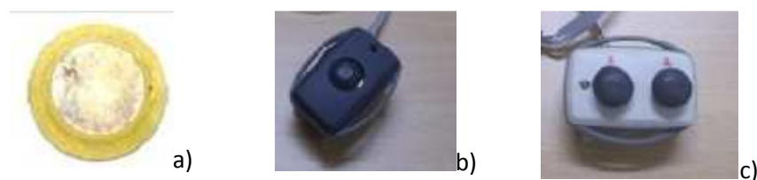
Figure 2.11 – a) A MuRata® PZ sensor, b) single and c) double headed probe.
