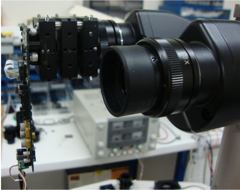
Figure 35 - Picture of the CCD Camera mounted on the eyepiece.
