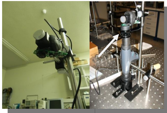
Figure 22 – The experimental set-up using the eyepiece (white arrow) at 6 centimetres from Panoptic™. The great field-of-view is re-established; however the image is not erect.
