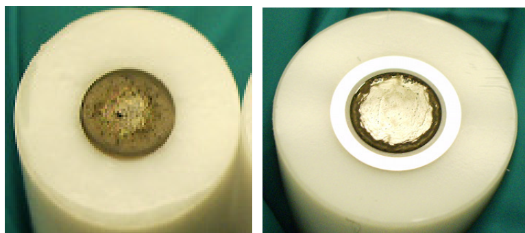
Figure 3.17 – RDE layers of a 2% Co/C2 catalyst. On the left the ink composition with 10% Nafion, on the right 1.7% Nafion was added to the ink solution.
