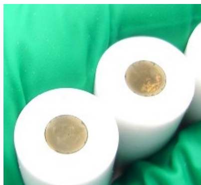
Figure 3.6 – RDE layers of a 38%Pt/C1 catalyst, 0.019 mgPt cm -2 (1.7% Nafion).
