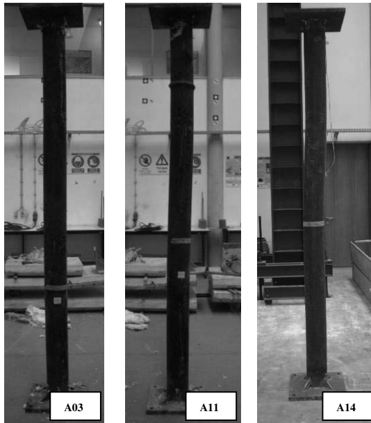
Figure 5. Columns totally filled with concrete (on left), with ring of concrete inside of 40mm (on center) and without concrete (on right), tube dia. = 168.3mm and load level = 30% N_{b,rd}
