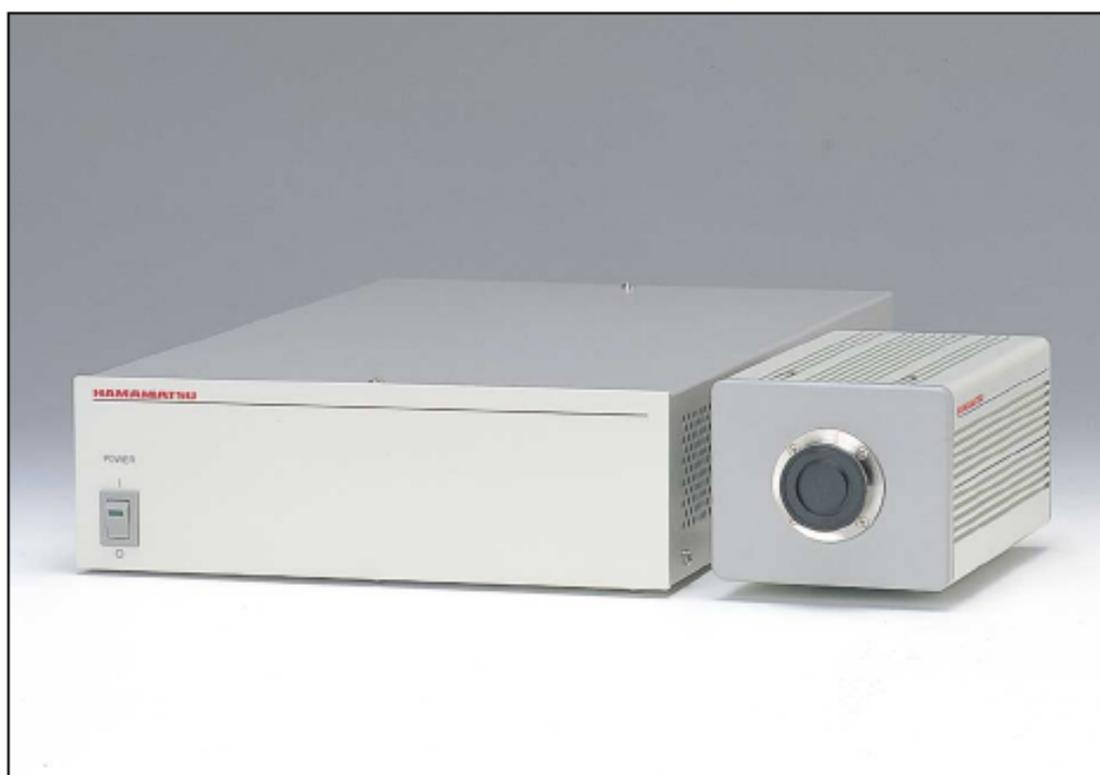
The ORCA-285 is a high resolution digital camera using a progressive scan interline CCD chip with no mechanical shutter. In addition to a high resolution of 1.37 million pixels, a wide dynamic range of 12 bit digital output and high sensitivity offers a wide application range down to low light level imaging.
