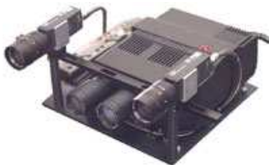
Figura 1.21: O C3D-2030 (de C3D/Edinburgh Virtual Environment Centre) – um sistema de scanning 3D multi-ocular [C3D/Edinburgh Virtual Environment Centre].
