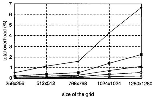
Fig. 3 Total overhead of NBC with different checkpoint intervals (ISING)
