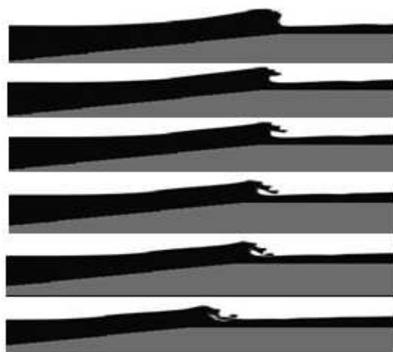
Figure 4.30 - Wave shape on the reef with a submergence of 1.5 m (after 63 s, wave 3).
