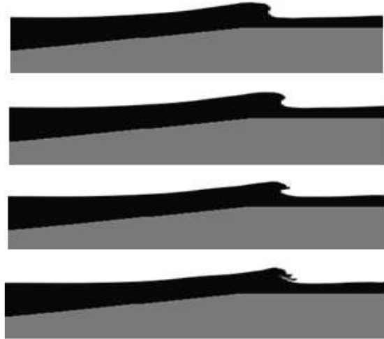
Figure 4.31 - Wave shape on the reef with a submergence of 2.0 m (after 63 s, wave 3).
