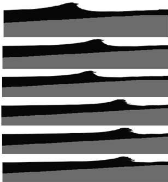
Figure 4.24 - Wave shape on the reef with a slope of 1:18 (after 62 s, wave 3).
