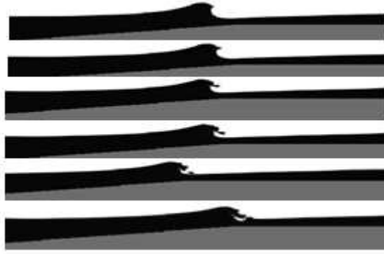
Figure 4.23 - Wave shape on the reef with a slope of 1:14 (after 91 s, wave 6).
