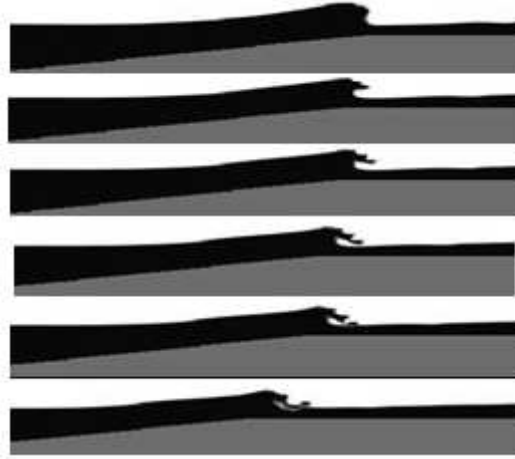
Figure 4.17 - Wave shape on the reef with a height of 3.20 m (after 62 s, wave 3).
