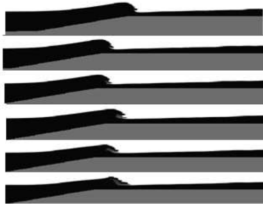
Figure 4.21 - Wave shape on the reef with a slope of 1:6 (after 62 s, wave 3).
