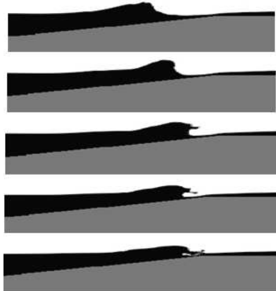
Figure 4.28 - Wave shape on the reef with a submergence of 0.8 m (after 63 s, wave 3).
