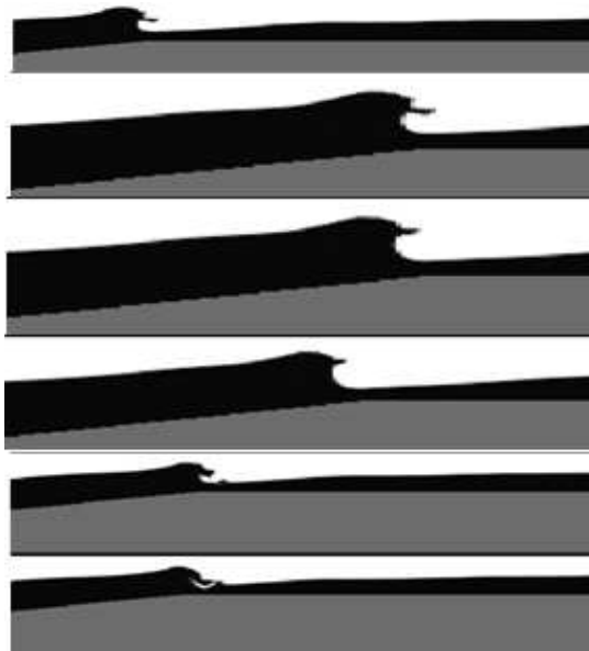
Figure 4.16 - Wave shape on the reef with a height of 3.90 m (after 62 s, wave 3).
