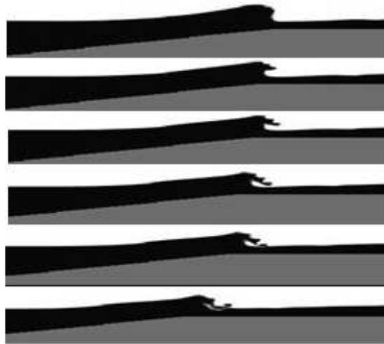
Figure 4.22 - Wave shape on the reef with a slope of 1:10 (after 62 s, wave 3).
