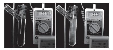
**Figure 2.** Supercooled water. A test tube with bidistilled water was introduced into a receptacle containing a mixture of saturated salted water and ice below the freezing point (on the left). When crystallization occurs, the temperature increases to  $0 \,^{\circ}$ C (on the right).
