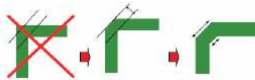
Figure 40 – Poor and good right angle bends - 2 corners of 45° should be used instead of the right angle corner.
