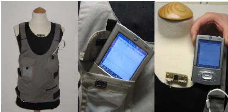
Figure 5 - The Vital Jacket - The system consists of a waistcoat in which the biosensors are integrated (left image). Data are wirelessly sent to a PDA for visualization and analysis (centre and right images). [17]
