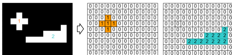
Illustration 44 - Connected pixels labelling algorithm working representation.
