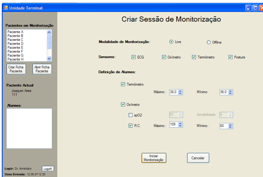
Figure 16: The creation of monitoring session with the possibility of managed the desired sensors and the alarms definitions.
