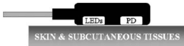
Fig. 5: A scheme of the typical reflectance probe organization and placement.[11]
