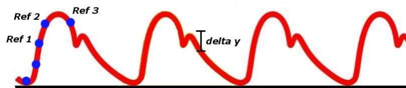
Grap. 10: Errors associated to the \Delta_y definition, in this case the Ref 2 would be mistakenly considered a maximum.
