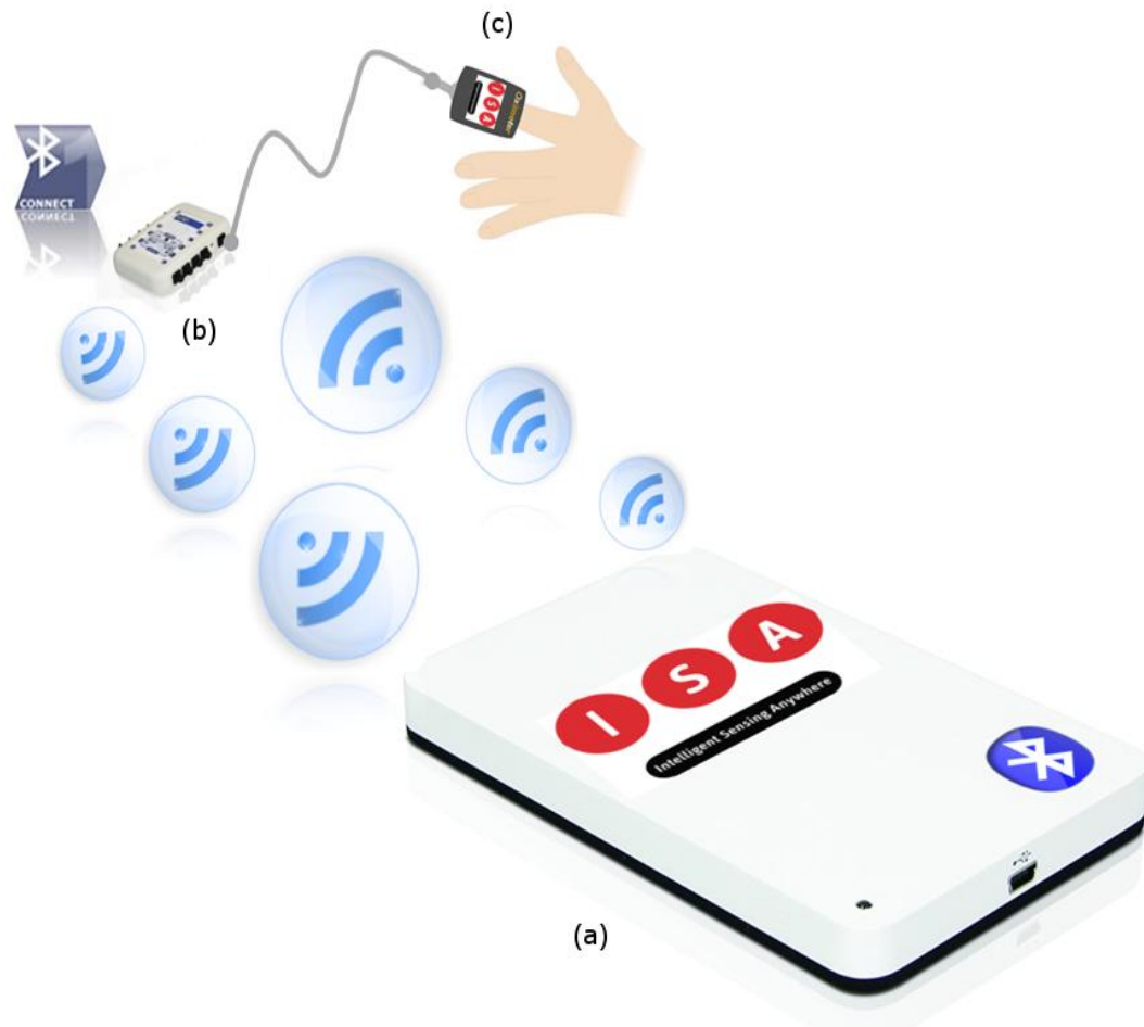
Fig. 21: The final system architecture: (a) Leonardo ® board, (b) Bioplux ® module and (c) transmittance oximetry probe.
