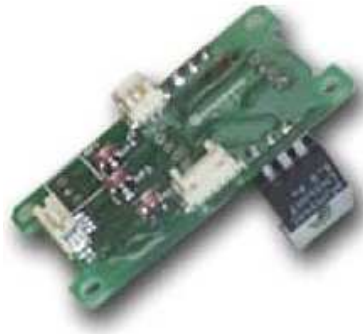
Figure 5.13. Driver Board, the hardware actuation of the proportional valve, from Kelly Pneumatics. From [36]
