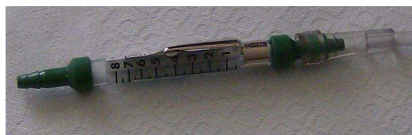
Figure 7.8. The flow meter.
