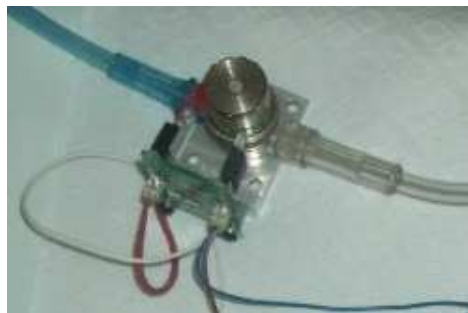
Figure 7.7. The electronic proportional valve with the tube (blue) placed in the gateway and the flow meter in the output port (white).
