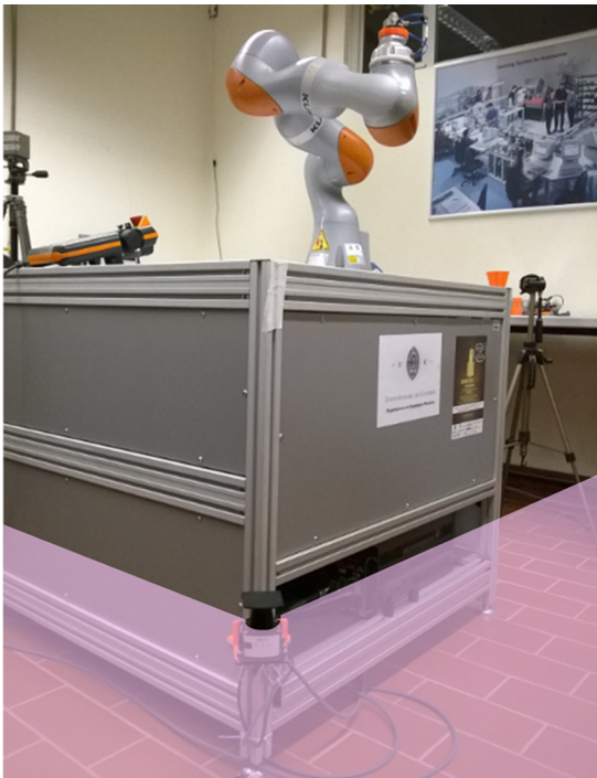
Fig. 2. Laser scanner mounted at the level of the operator's legs in the base of the robot table. If the robotic arm is installed on a mobile platform the solution is similar.
