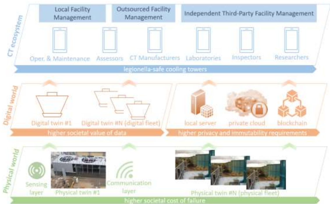
Fig. 6: Legionella-safe cooling tower: ecosystem design.
