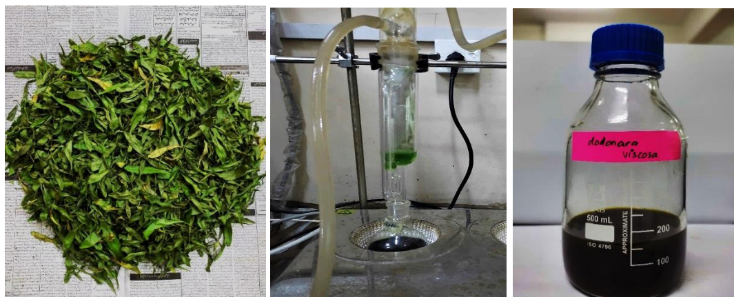
Figure 4.1. Dried leaves of Dodonaea viscosa (Left). Soxhlet extraction of plant phytochemicals (Middle). Prepared ethanolic extract of Dodonaea viscosa (Right).
