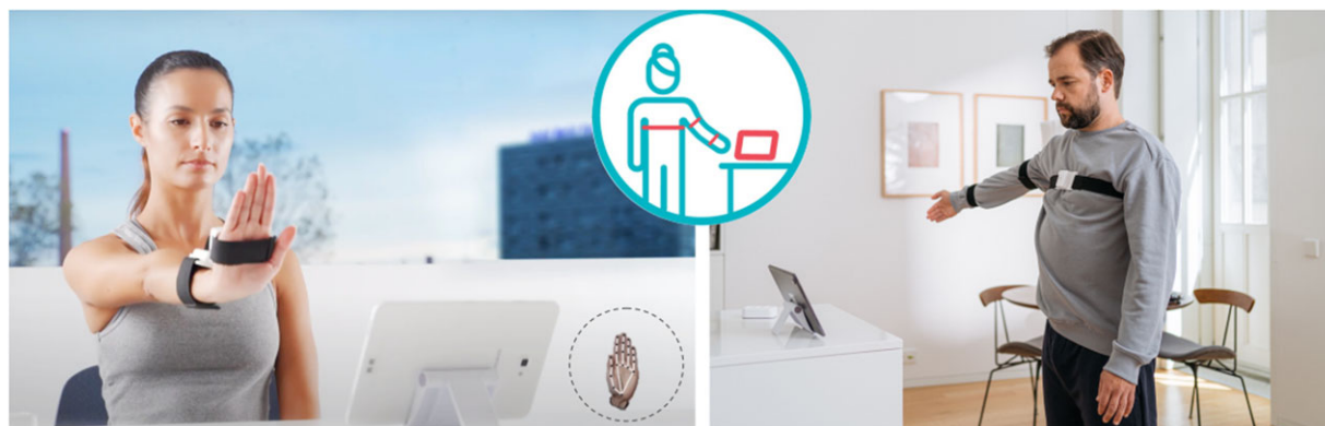
Figure 1. Motion trackers positioning for hand/wrist (in this case camera-vision is also applied to track movements) (left image) and for shoulder and elbow (right image).
