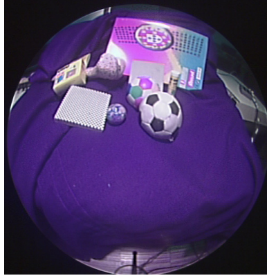
Figure 5.3: Scene acquired with an Arthroscopic Camera. The lens used induce strong radial distortion in the image.
