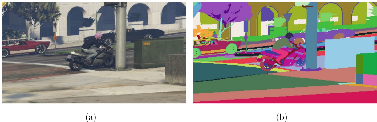
Figure 2.2: RGB image (a) and equivalent raw semantic segmentation map (b) obtained from GTA V virtual environment. From [29].
