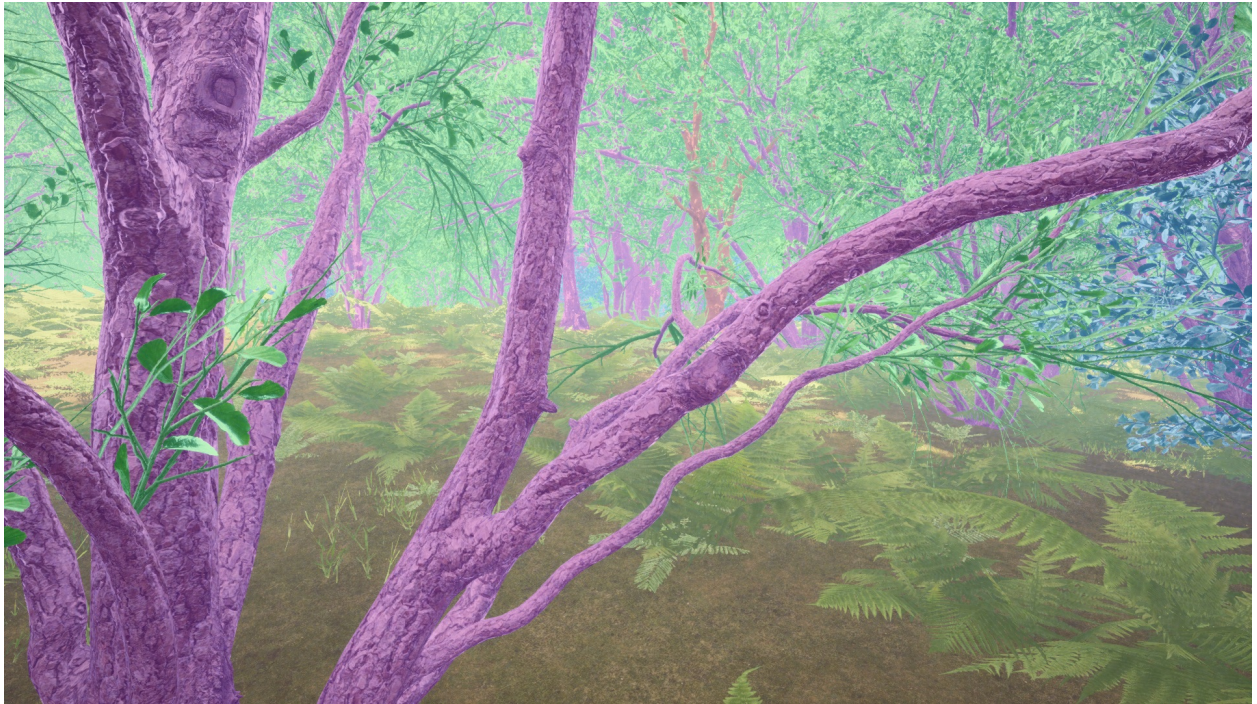
Figure 5.3: Example of semantic segmentation maps precision verification. Layering of the RGB and semantic segmentation map images, with opacity at 100% and 25%, respectively.
