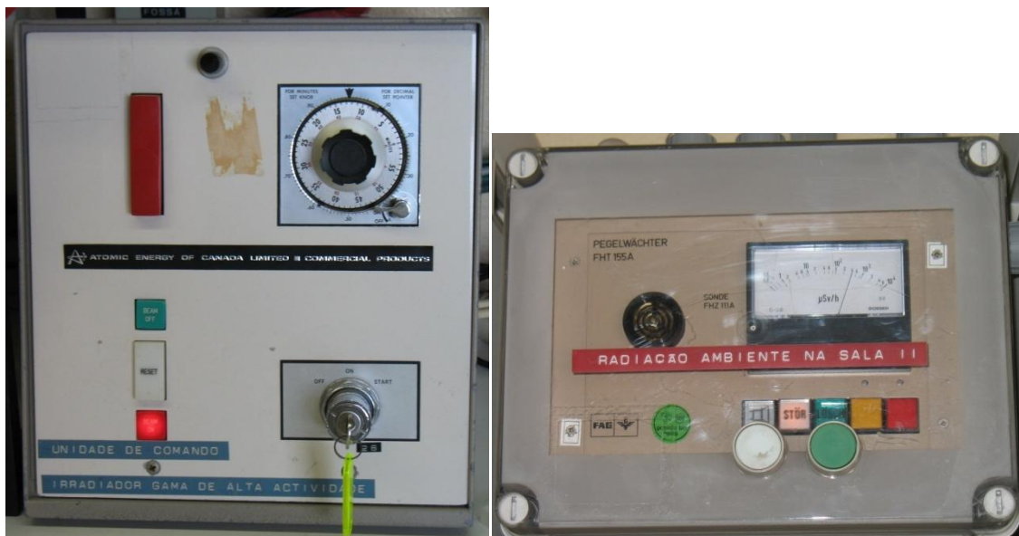
Fig. 15 - Left: Irradiator command unit. Right: Environmental dose equivalent monitor performs readings inside irradiation bunker.
