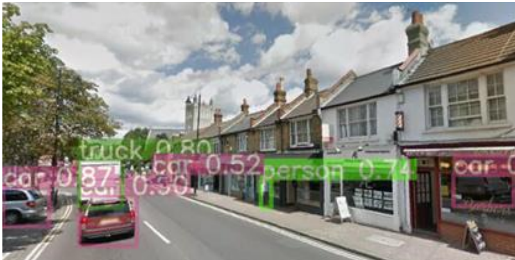
Figure 7. Example of a GSV image after executing YOLOv5.
