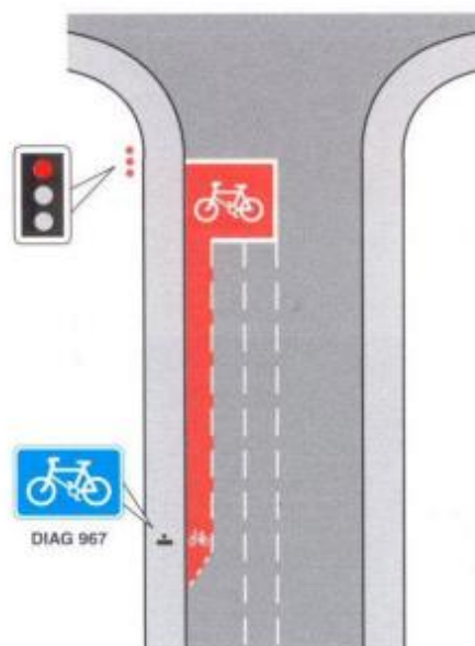
Figure 2. Schematic layout of advanced stop line [61].
