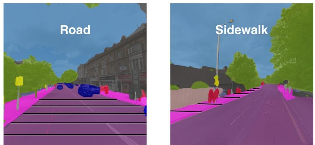
Figure A4. Example illustrating the potential of IS to extract road (left) and sidewalk (right) width.
