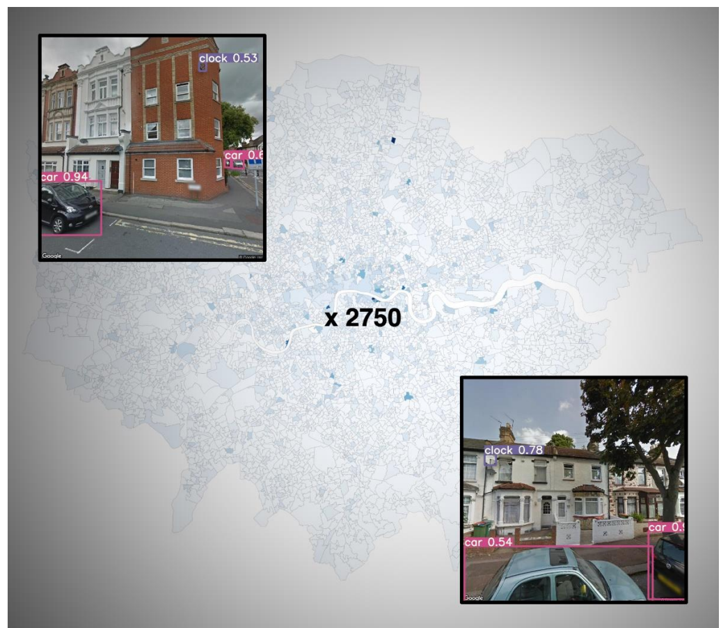
Figure A2. Example of misclassification in YOLOv5.
