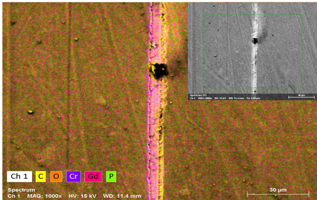
Figure 12. EDS of 2.3% Gd-DLC with IL#1 and SEM image of the same in top right corner.
