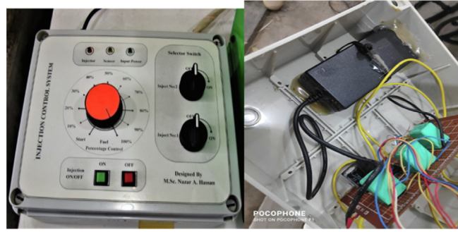
Fig. 3 The control mechanism for LPG injection.
