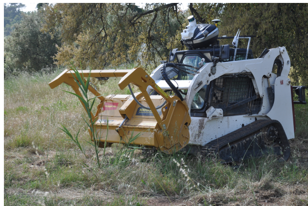
Figure 1. SafeForest Unmanned Ground Vehicle (UGV), showing the sensor system (including LiDAR, RGB, and depth cameras on the top of the vehicle) and the vegetation cleaning attachment at the front.
