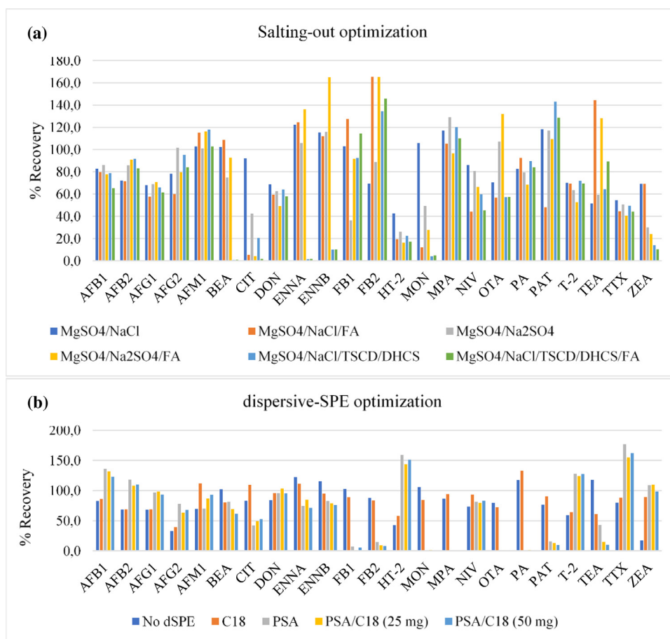
Fig. 4. Recovery values, in percentage, for analysis of different (a) salting-out reagents, and (b) modified-QuEChERS methods, concerning dispersive-SPE step.
