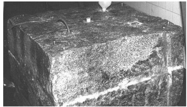
Fig. 2. Granite block and detail of the sealed fracture.
