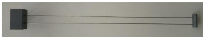
Figura 4.13 - Sonda twin wire
