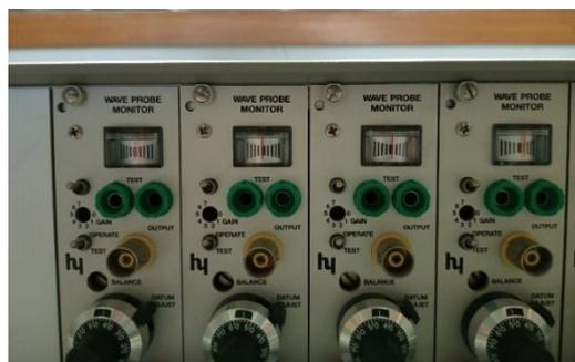
Figura 4.19 - Wave probe monitor
