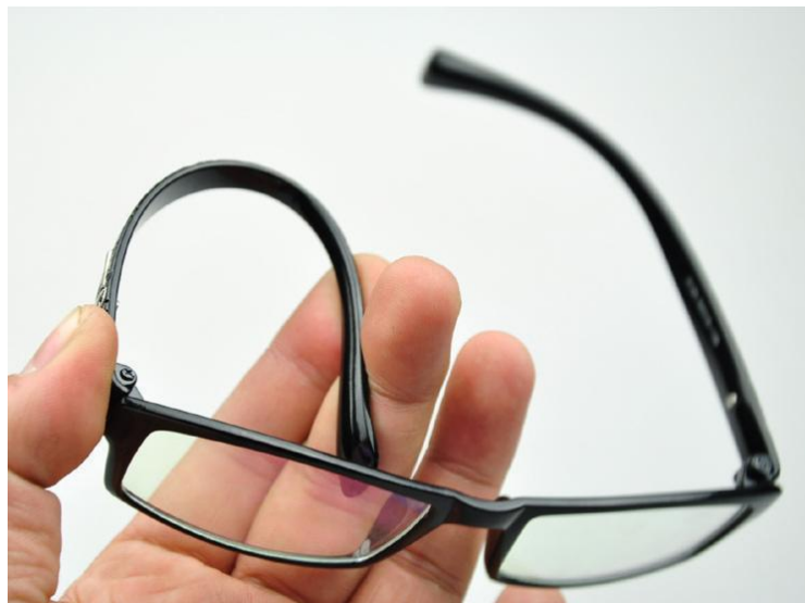
Figure 6- Glasses made of a SMA showing the superelasticity effect.
