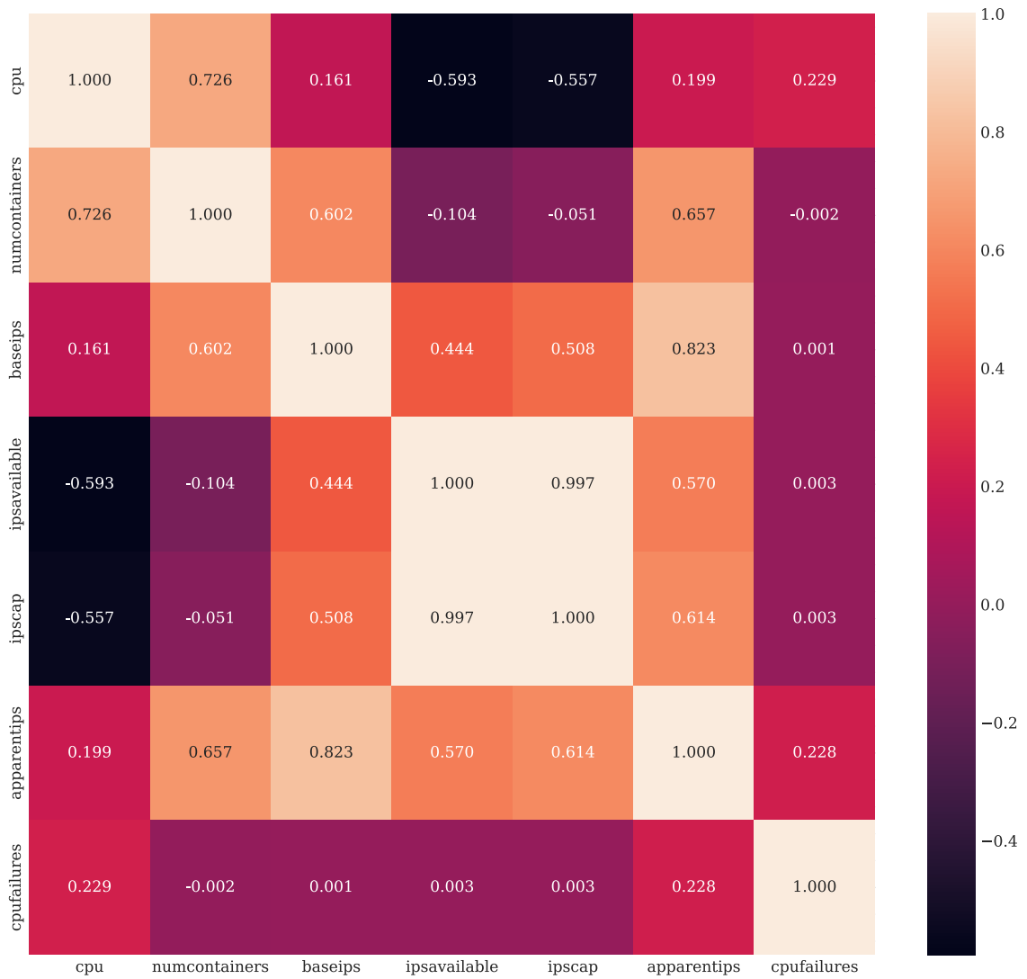
Figure 6.7: Correlation matrix of the CPU metrics collected from the hosts in scenario 1.
