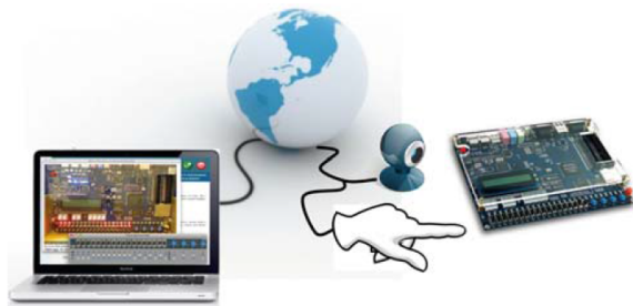
Figure 7. Concept of the reconfigurable logic remote laboratory board: virtualised board keys and switches, webcam to observe LEDs, 7 segment displays and LCD display [5,6].
